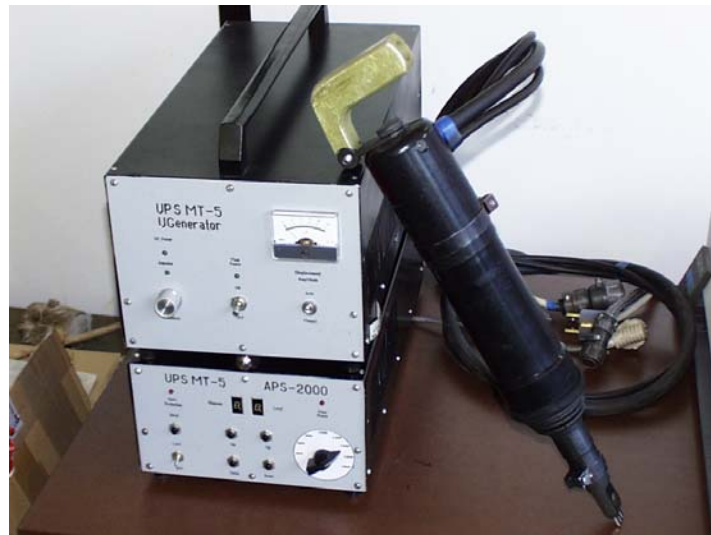
FIGURE 1. The 27 kHz ultrasonic impact treatment equipment.
