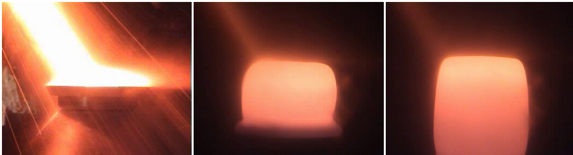
FIGURE 1. Three subsequent stages during spray forming of the billet.
