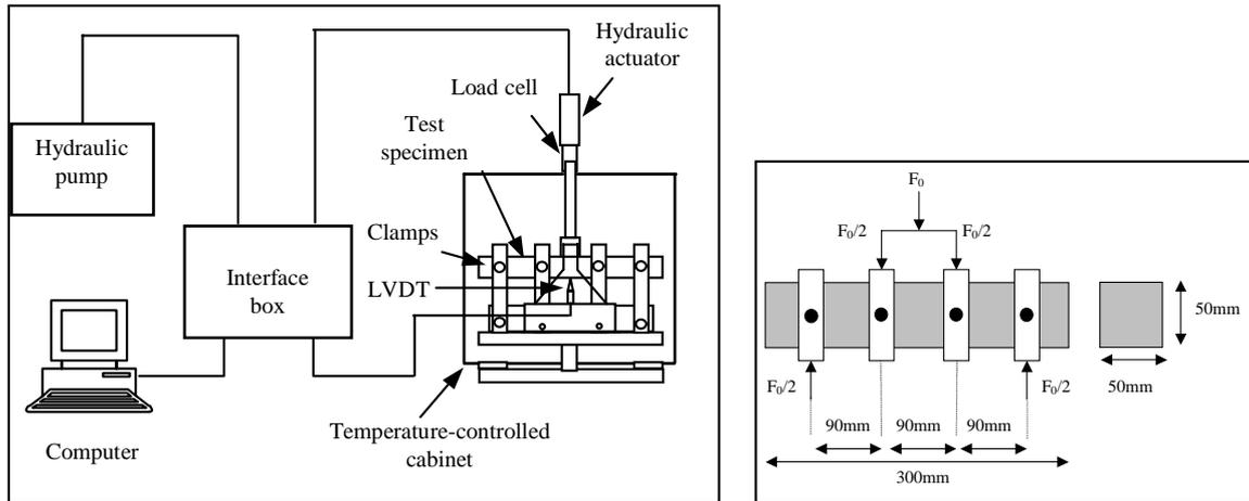
FIGURE 1. 4PB test apparatus and test configuration
