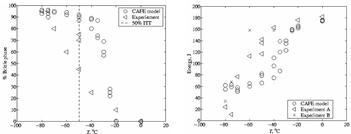
FIGURE 6. Percentage of brittle phase and transition Charpy energy data. The 50% ITT and experimental data A are taken from Bhattacharjee et al. [13]; the experimental brittle phase was provided by Corus UK Ltd and the experimental data B is courtesy of Davis [14].
