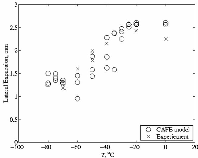
FIGURE 7. Simulated and experimental Charpy lateral expansion data.
