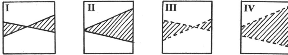
FIGURE 2. The four grain boundary failure mechanisms. The boundary is shown schematically as a square and the parts which must fail are indicated by shading, the straight edges of which are the traces of the two cleavage planes. In mechanisms I and II the crack crosses the boundary whereas in III and IV two cracks meet the boundary from opposite sides.
