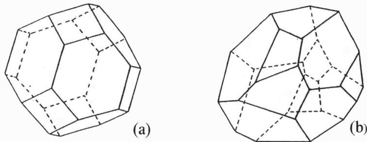
FIGURE 4. Individual grains of model 3-d polycrystals: (a) the regular 14-hedron, (b) a randomly generated polyhedron with 16 faces. The bold lines represent faces on the front of the model and the broken fine lines those on the back.
