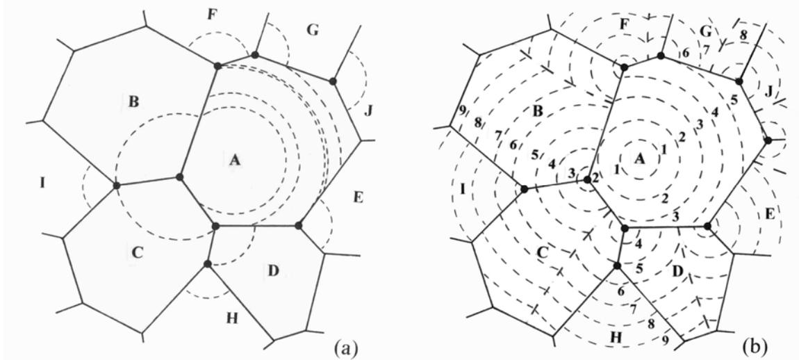
FIGURE 3. Cross-sections of a few grains of a model pseudo 3-d polycrystal. A cleavage crack nucleates in grain A and propagates into neighbouring grains at the sites on grain edges indicated by dots. In (a) only one crack is allowed in each grain but in (b) two parallel cracks from two different edges may nucleate and give rise to stepped cleavage planes, time increments being indicated by numbered broken circles and possible steps by bold slightly curved broken lines.
