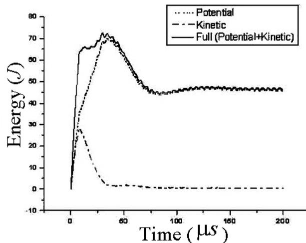
FIGURE 6. Transmitted energy time dependence
