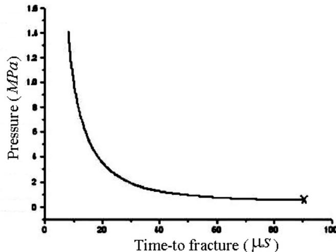
FIGURE 3. Curve limiting the pulses leading to crack propagation
