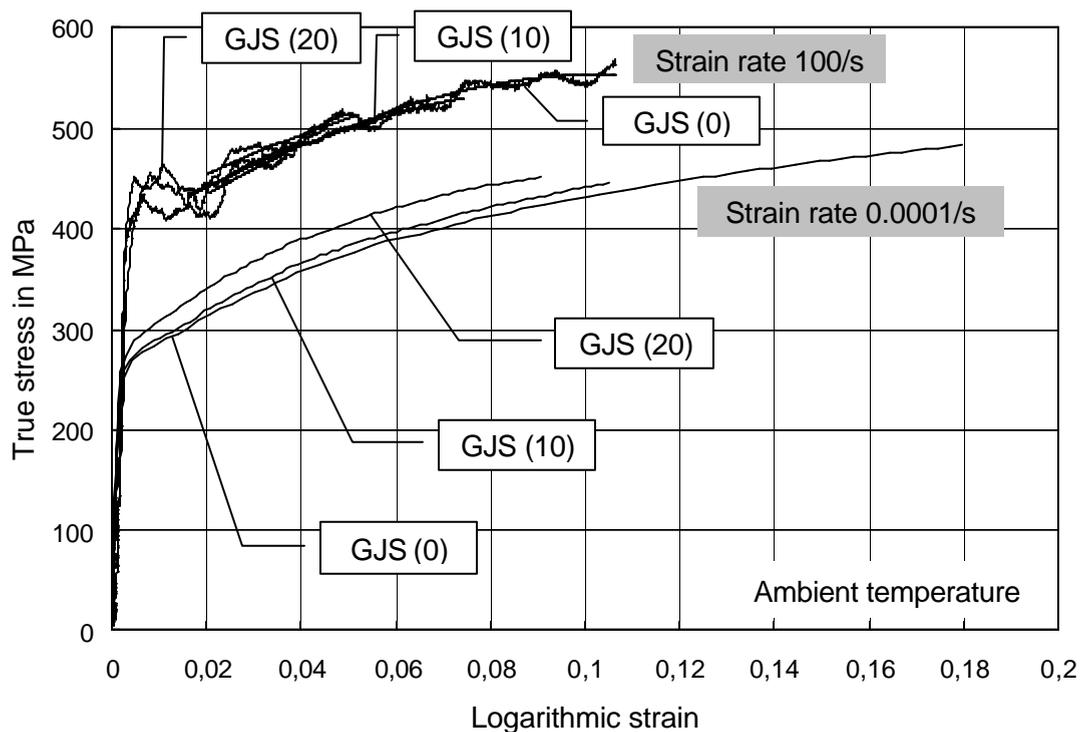
FIGURE 5. Influence of pearlite content on the true stress-strain behaviour of DCI at two selected strain rates, ambient temperature.
