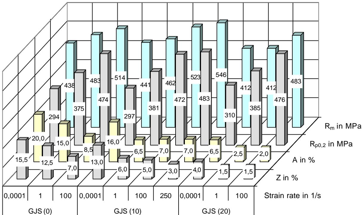
FIGURE 4. Strength and deformation characteristics of GJS (0), GJS (10) and GJS (20) for different strain rates at -40 °C.
