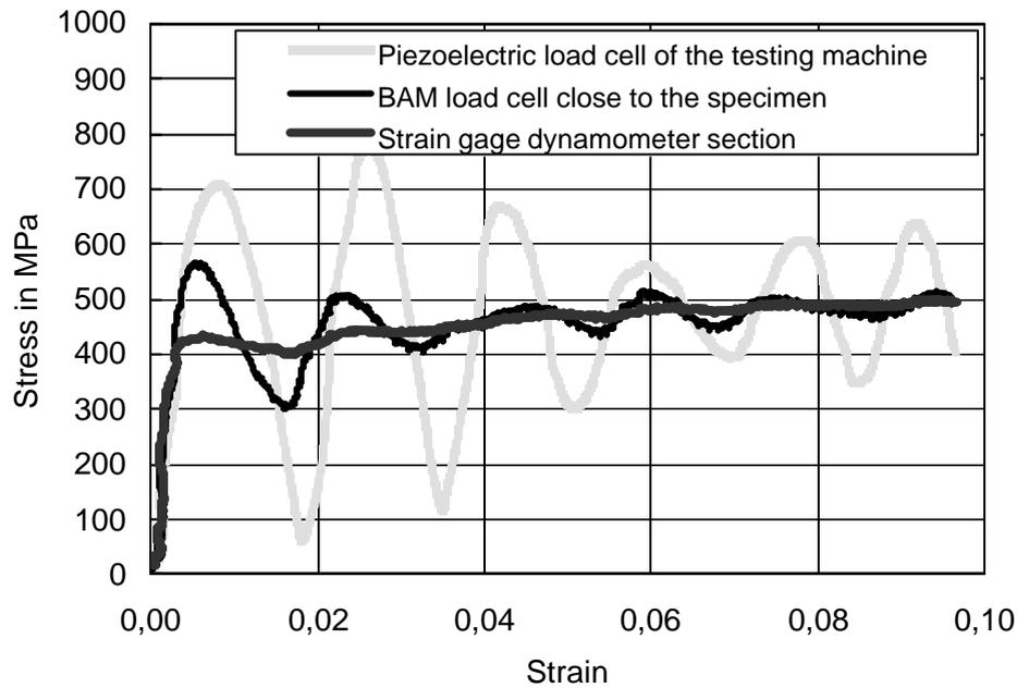
FIGURE 3. Force measurement techniques and resulting engineering stress-strain curves, GJS (0), ambient temperature, strain rate 100/s.
