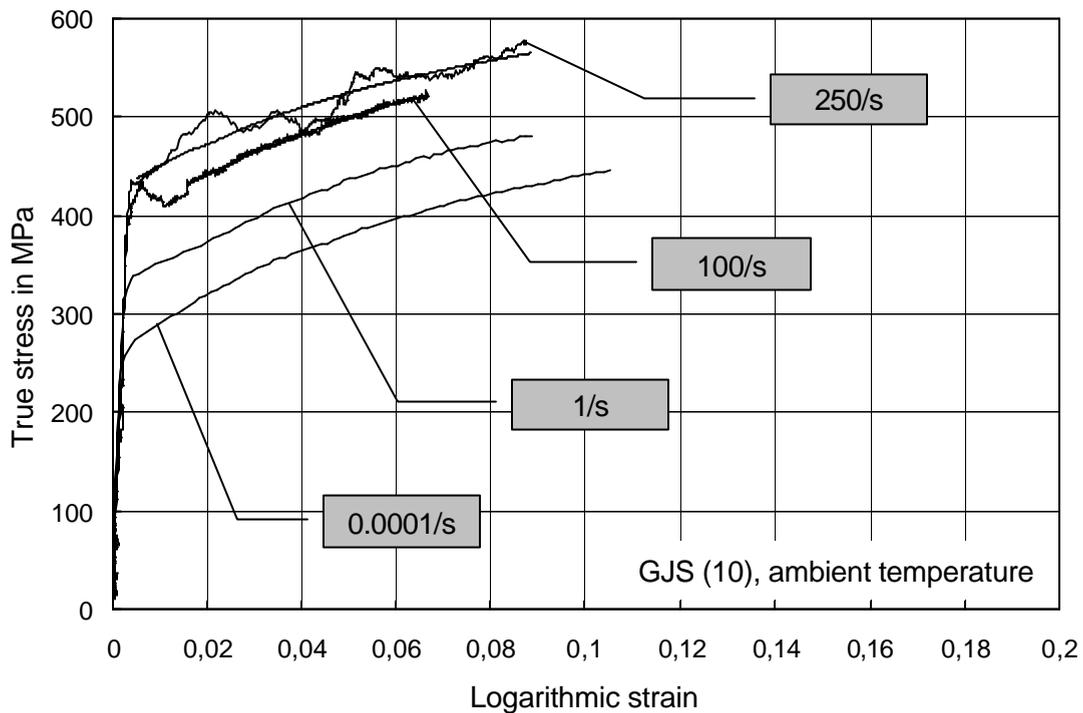
FIGURE 7. Influence of strain rate on the true stress-strain behaviour of DCI, GJS (10), ambient temperature.
