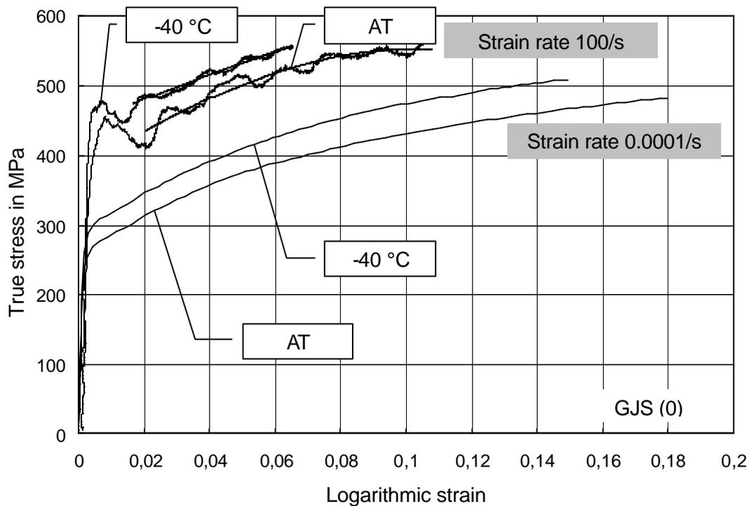
FIGURE 6. Influence of temperature on the true stress-strain behaviour of DCI at two selected strain rates, GJS (0), AT – ambient temperature.
