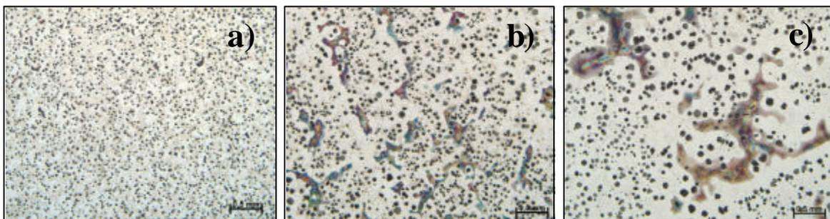
FIGURE 1. Metallographic images of the investigated DCI materials with pearlite content of 0 % (a), 10 % (b) and 20 % (c).
