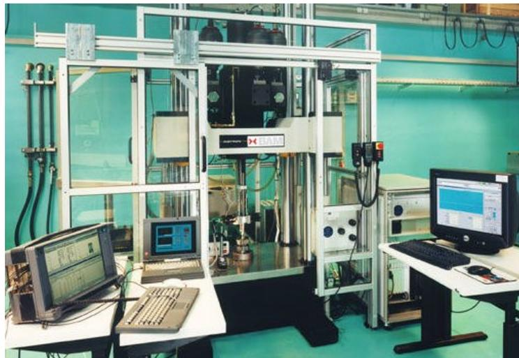
FIGURE 2. Servo-hydraulic high-speed test system, maximum force 50 kN, maximum piston speed 25 m/s.
