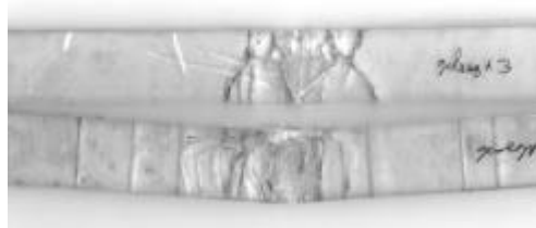
Figure 4 : Photo of layered glass (top) and segmented specimen after testing
