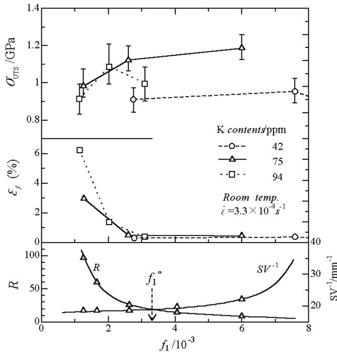
**Figure 7:** Variations of the ultimate tensile strength  $\sigma_{UTS}$  and the total elongation  $\epsilon_f$  with the grain morphology index  $f_1$  for doped wires annealed for 300 s at 2660 K after heating at the rates of 0.2-985 K/s.
