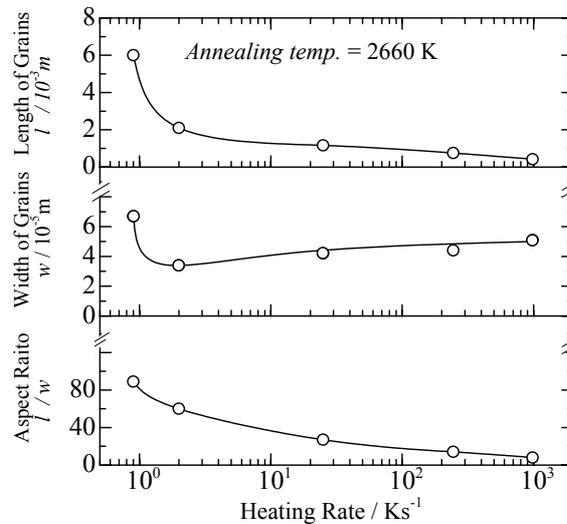
**Figure 1:** Variations of the length  $\ell$ , the width  $w$  and the aspect ratio  $R$  ( $=\ell/w$ ) of secondary recrystallized grains with heating rate for doped tungsten wire with a potassium concentration of 75 mass ppm.
