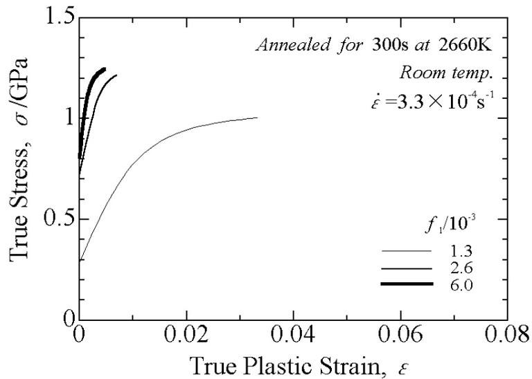
**Figure 5:** True stress-true strain curves for doped wire with a potassium concentration of 75 mass ppm.
