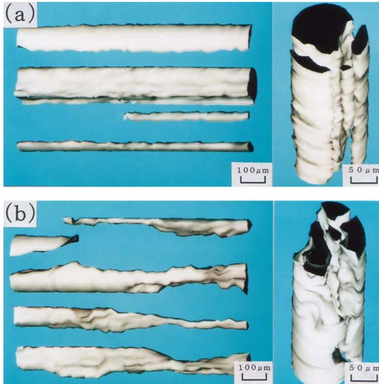
**Figure 2:** Stereoscopic views of secondary recrystallized grains for doped wire, which is annealed for 300 s at 2660 K after heating at the rates of (a) 0.5 and (b) 330 K/s, with a potassium concentration of 75 mass ppm.
