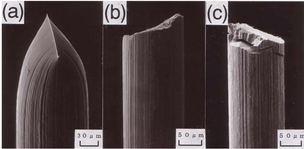
**Figure 6:** SEM photographs of fractured surface. The photographs (a) to (c) correspond to each specimen with a value of  $f_1/10^{-3} = 1.4, 3.3$  and  $6.0$ , respectively, in Figs.4 and 5.
