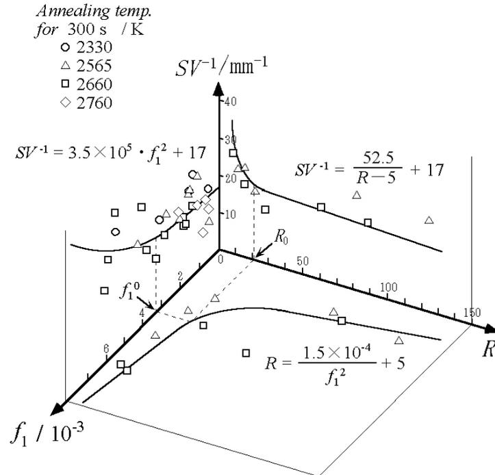
**Figure 3:** The relationship between the grain morphology index  $f_1$ , the grain aspect ratio  $R$  and the area of grain boundaries per unit volume of a specimen  $S/V$ . The critical value  $R_0$  indicates the minimum grain aspect ratio at which  $S/V$  begins to increase with a decrease in  $R$ .
