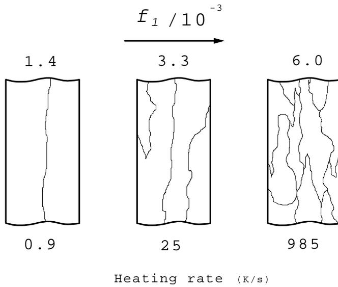
**Figure 4:** Schematic representation of the heating rate dependence of grain morphology expressed as a function of the grain morphology index  $f_1$ .
