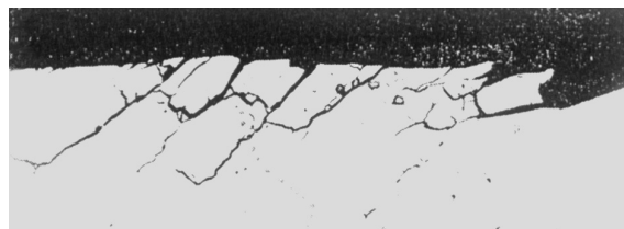
Figure 5: Cracking of the lubricated surface of roller from rail steel under contact fatigue testing [9].
