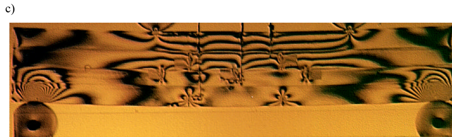
Figure 1: a) Four-layer beam with cracks. Photoelastic model under four point bending, the isochromatic patterns ( \sigma_1 - \sigma_2 ) distribution b) Initial loading ( P = 20.0 N). c) P = 50.0 N - tension of layers 2, 3 and 4.
