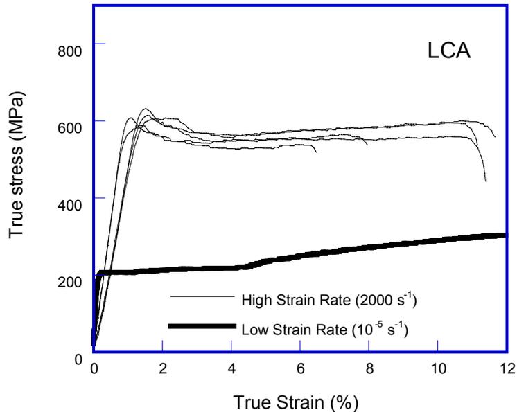
**Fig. 3:** Stress-strain curves obtained for LCA wires
