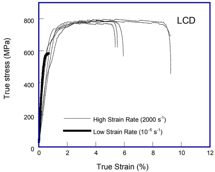
**Fig. 2:** Stress-strain curves obtained for LCD wires
