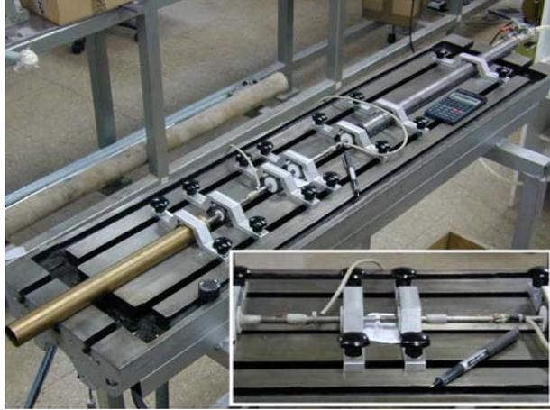
**Fig. 1:** Experimental testing device used in the high strain rate tests. Detail of the specimen location in the testing device.
