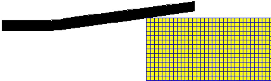
**Fig. 4:** Finite element mesh used for modelling of cold drawing.
