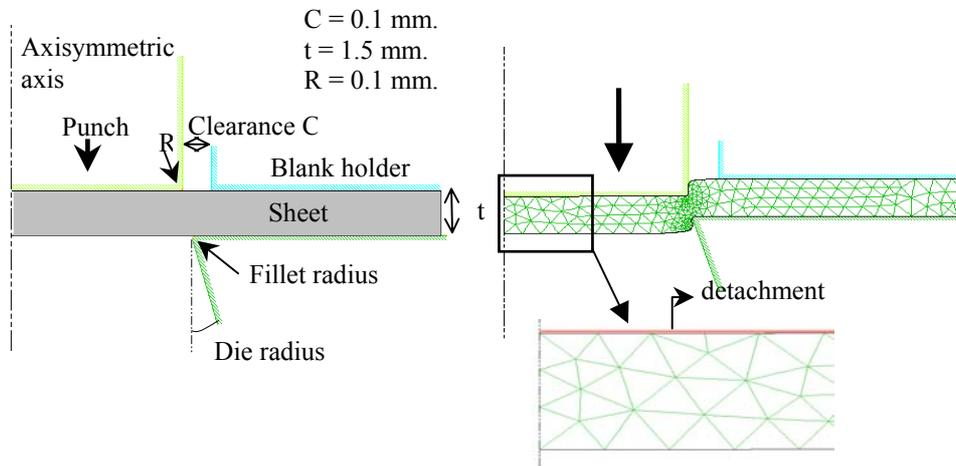
**Figure 2:** Numerical simulation of the cutting process
