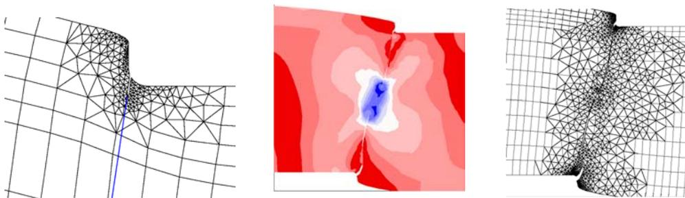
**Figure 7:** crack propagation during the cutting process, using the maximum shear stress criterion
