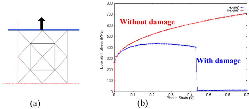
**Figure 3:** Uniaxial tensile test with coupled damage
