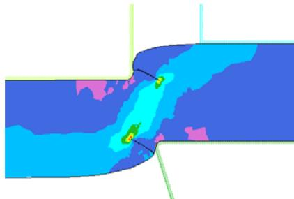
**Figure 6:** wrong crack path according to the maximum circumferential stress criterion during the cutting process.
