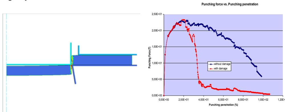
**Figure 4:** a) damage concentration during the cutting process b) comparison of load-displacement curves.
