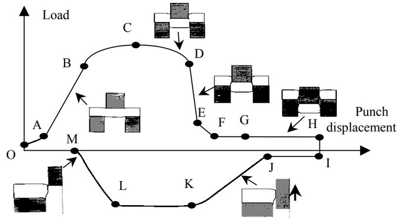
**Figure 1:** Load-displacement curve of the cutting process.
