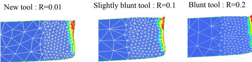
**Figure 5:** influence of the sharpness of the cutting tool on the cut edge morphology.
