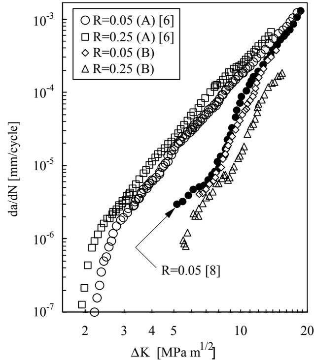
**Figure 1:** Fatigue crack growth rates for 6082-T6 aluminium alloys.
