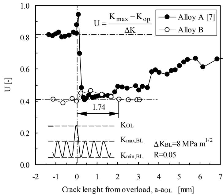
**Figure 4:** Crack closure response following a single tensile overload.
