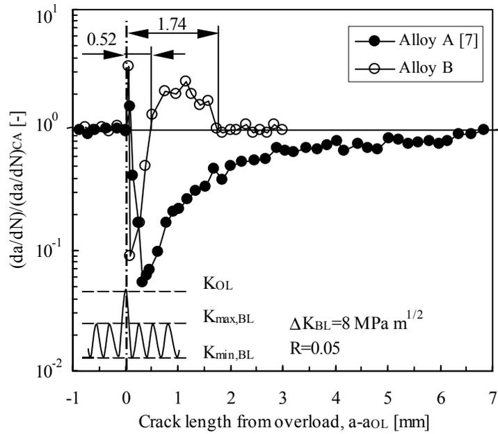
**Figure 3:** Transient crack growth rate following a single tensile overload.
