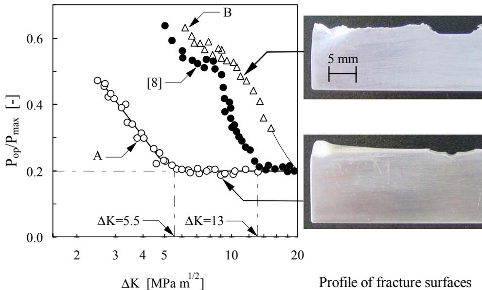
**Figure 2:** Crack closure data and profiles of fracture surfaces for 6082-T6 alloys. R=0.05
