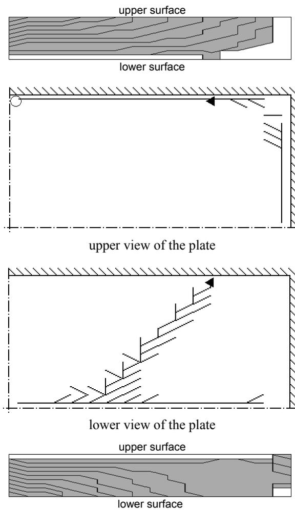
**Figure 1:** Surface cracking at time  $t_2$ .
