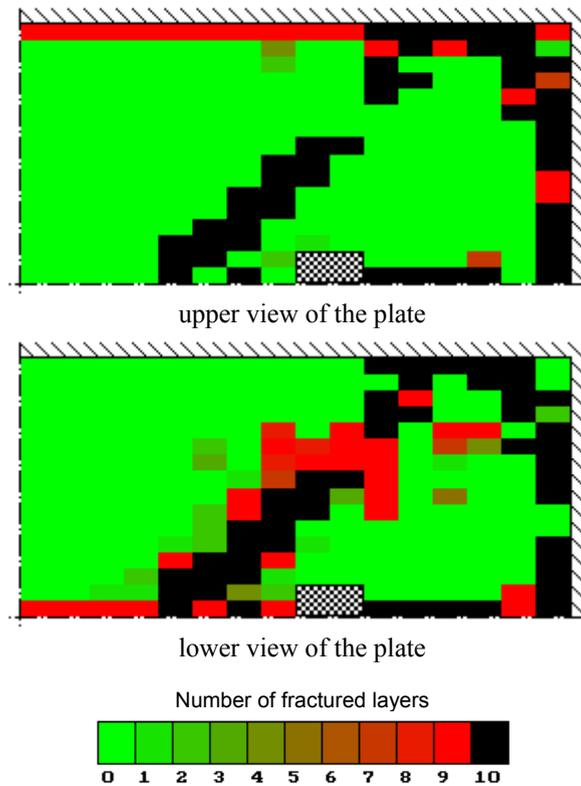
**Figure 2:** In-deep penetration of cracks at time  $t_3$ .
