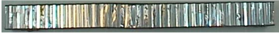
Figure 6: Photograph of sandwich beam with aluminum honeycomb core impacted from 127 mm height, showing debonding and distortion of the specimen.
