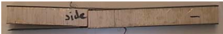
Figure 5: Photograph of sandwich beam with balsa wood core impacted from 254 mm height, showing core failure and debonding.
