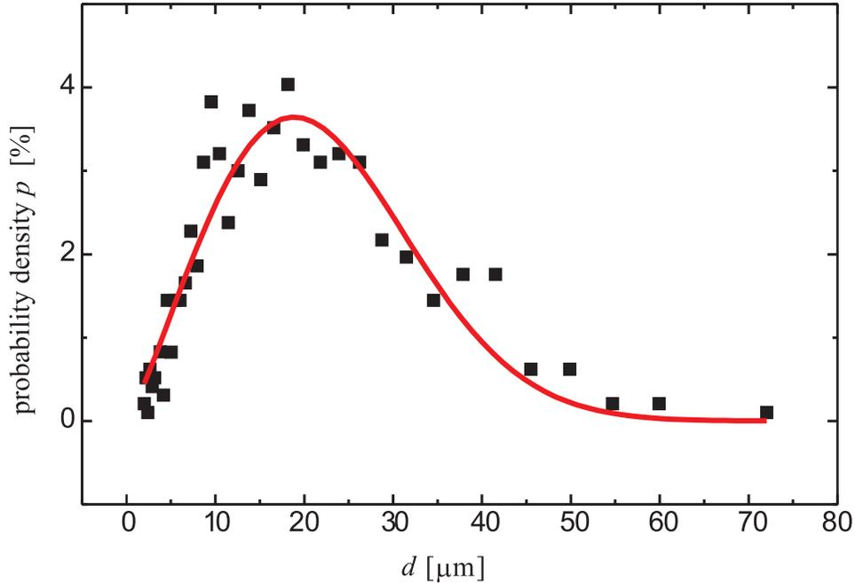
**Figure 3:** Weibull fit of experimental grain size data for ARMCO iron ( $d_m = 20 \mu\text{m}$ )
