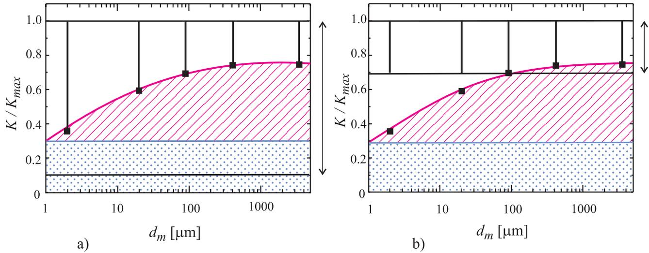
**Figure 5:** Scheme of the crack closure during the loading cycle with a)  $R = 0.1$ ; b)  $R = 0.7$ . Within the shadowed area the crack is closed. The hatched part shows the amount of RICC contribution
