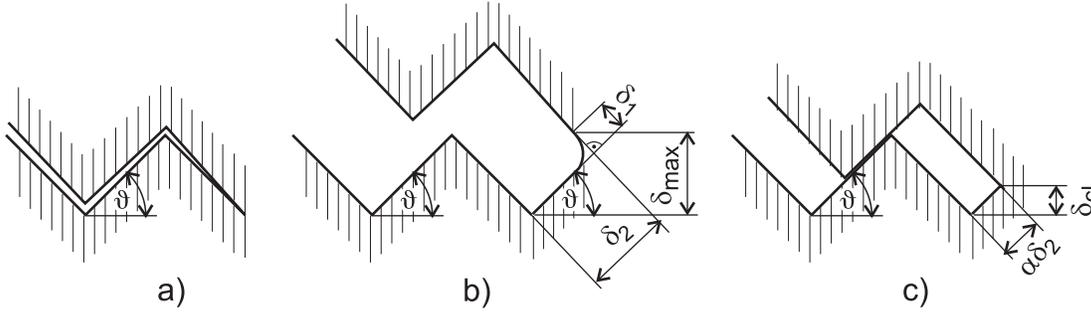
**Figure 2:** Scheme of the roughness induced crack closure mechanism
