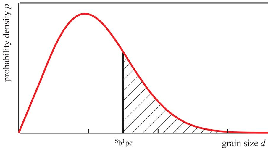
**Figure 1:** The dashed area under the probability density function corresponds to the relative number of grains involved in the roughness induced crack closure process
