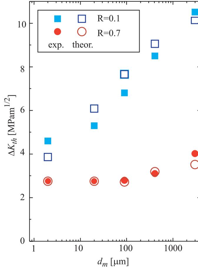
**Figure 4:** Comparison of experimental [6] and theoretical (Eqn. 8) data on threshold behaviour of ARMCO iron with different mean grain size
