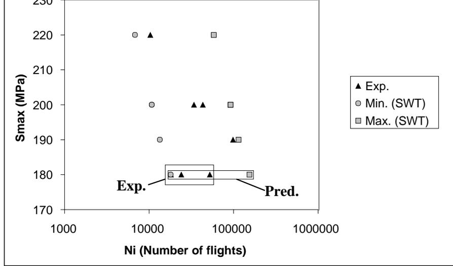
Figure 5: Predicted scatter for the 2<sup>nd</sup> spectrum, Smith-Watson-Topper correction.
