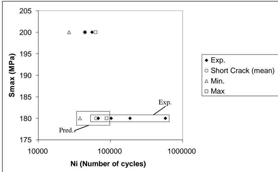
Figure 2: Predicted scatter for the CA conditions,  $R = 0.1$ , Short Crack approach.
