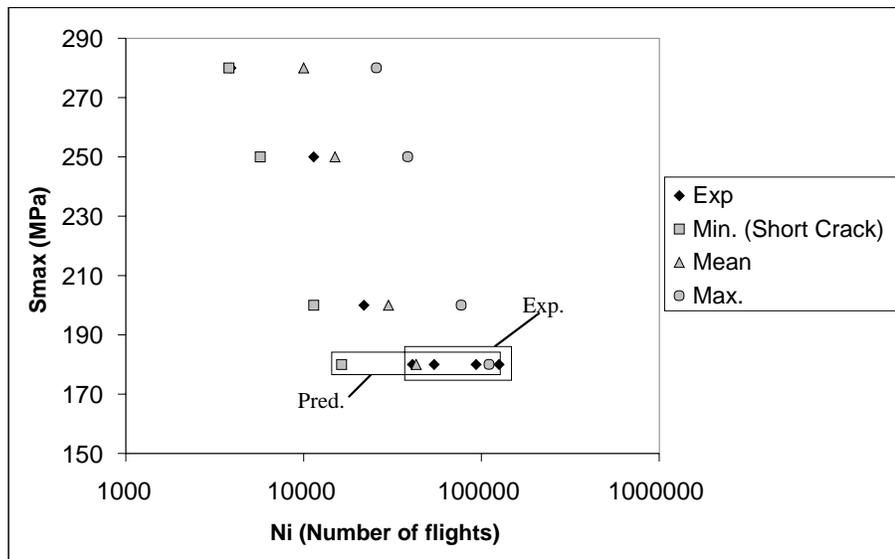
Figure 3: Predicted scatter for the 1<sup>st</sup> spectrum, Short Crack approach.
