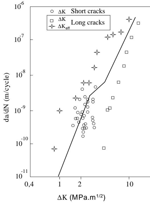
Figure 1: Experimental data and mean crack propagation law (Al 2024-T3, Desforges [8]).
