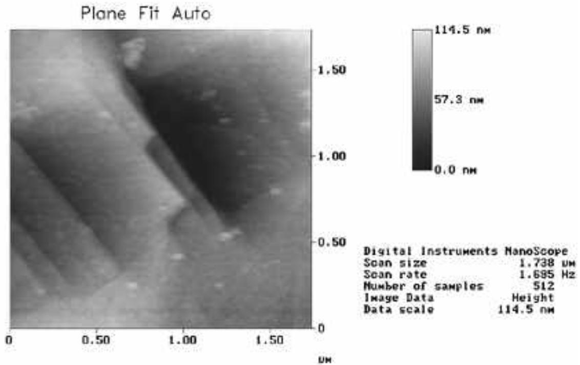
**Figure 8:** AFM observation at high magnification of slip bands and microcracks in  $\alpha$  platelets
