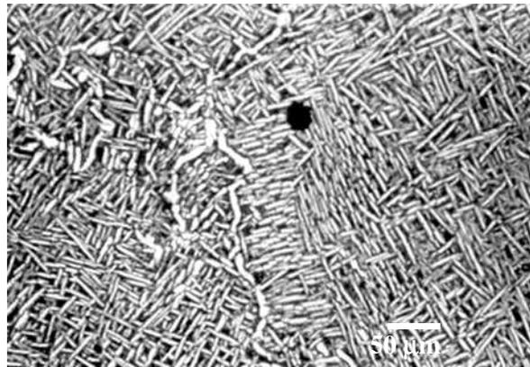
**Figure 1:** Microstructure of the Ti6246 alloy
