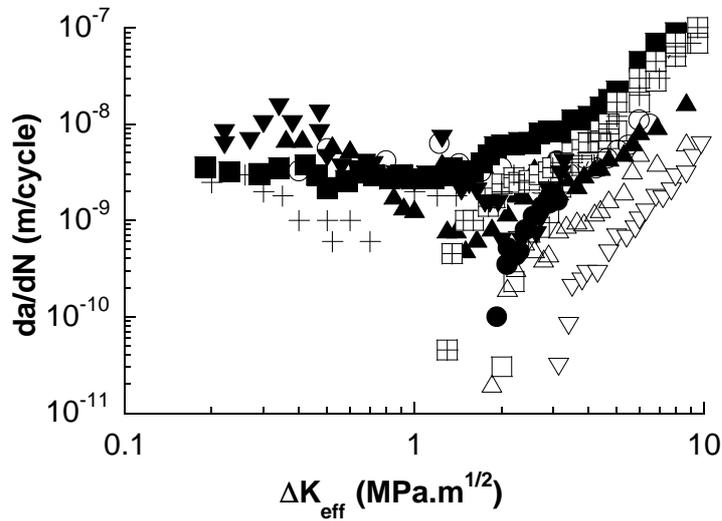
**Figure 3 :** Compilation of experiments demonstrating the existence of no-threshold behavior in various Ti alloys called the Marci effect at room or moderate temperature
