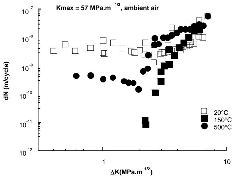
**Figure 4 :** Comparison of propagation curves obtained in air, at room temperature, 150°C and 500°C for  $K_{max} = 57 \text{ MPa}\sqrt{\text{m}}$
