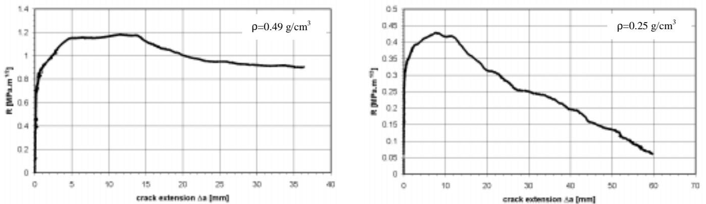
**Figure 5:**  $K_R$  vs.  $\Delta a$  curves of ALPORAS foam CT-specimens ( $W=290$  mm) with two different densities (same specimens as shown in Fig. 4).
