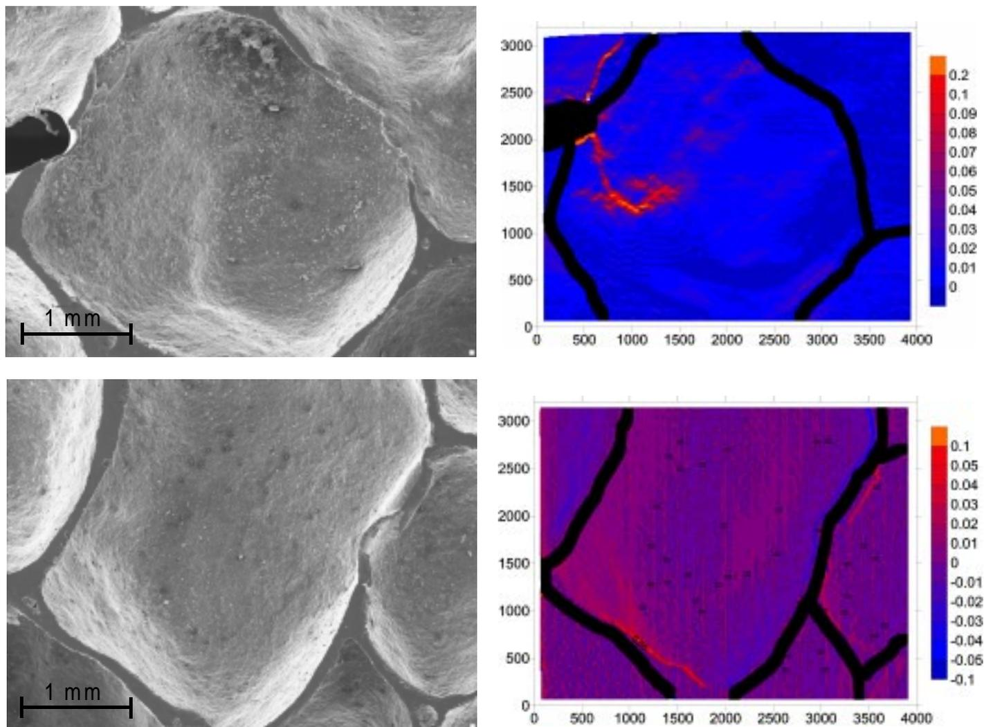
**Figure 7:** Measured local deformations at crack initiation in the first cell wall in front of the notch root (first row) in loading direction and in a cell in the center of the ligament (second row) perpendicular to the loading direction. 4000 pixels are equivalent to 3.3 mm.
