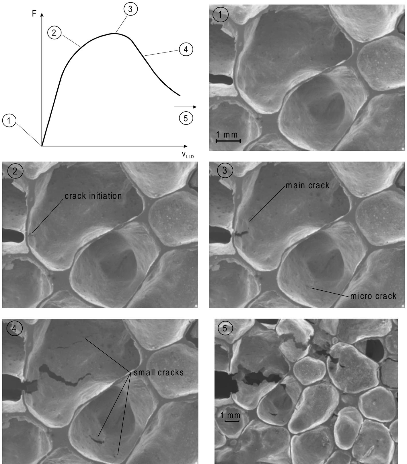
**Figure 6:** Schematic load vs. load line displacement curve with loads marked from these SEM micrographs were taken. ALPORAS foam,  $W=50$  mm,  $\rho=0,25$  g/cm<sup>3</sup>, description see text.
