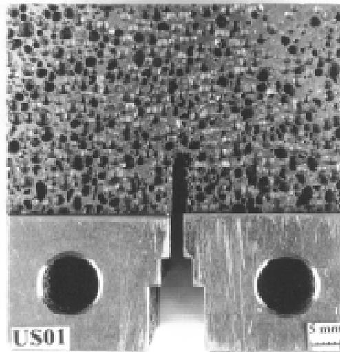
**Figure 1:** Example of a CT-specimen, which was used for the fracture tests.
