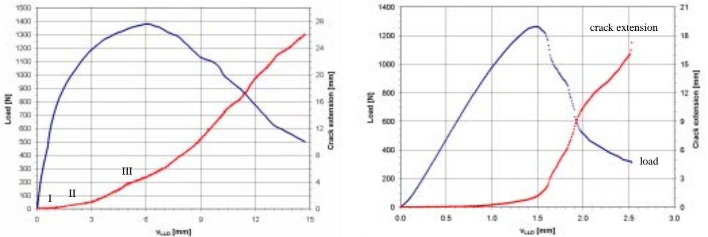
**Figure 2:** Load versus load line displacement curve and crack extension curve for an ALPORAS foam ( $W=140$  mm,  $\rho=0,45$  g/cm<sup>3</sup>) on the left side and for an ALULIGHT foam ( $W=100$  mm,  $\rho=0,50$  g/cm<sup>3</sup>) on the right side.
