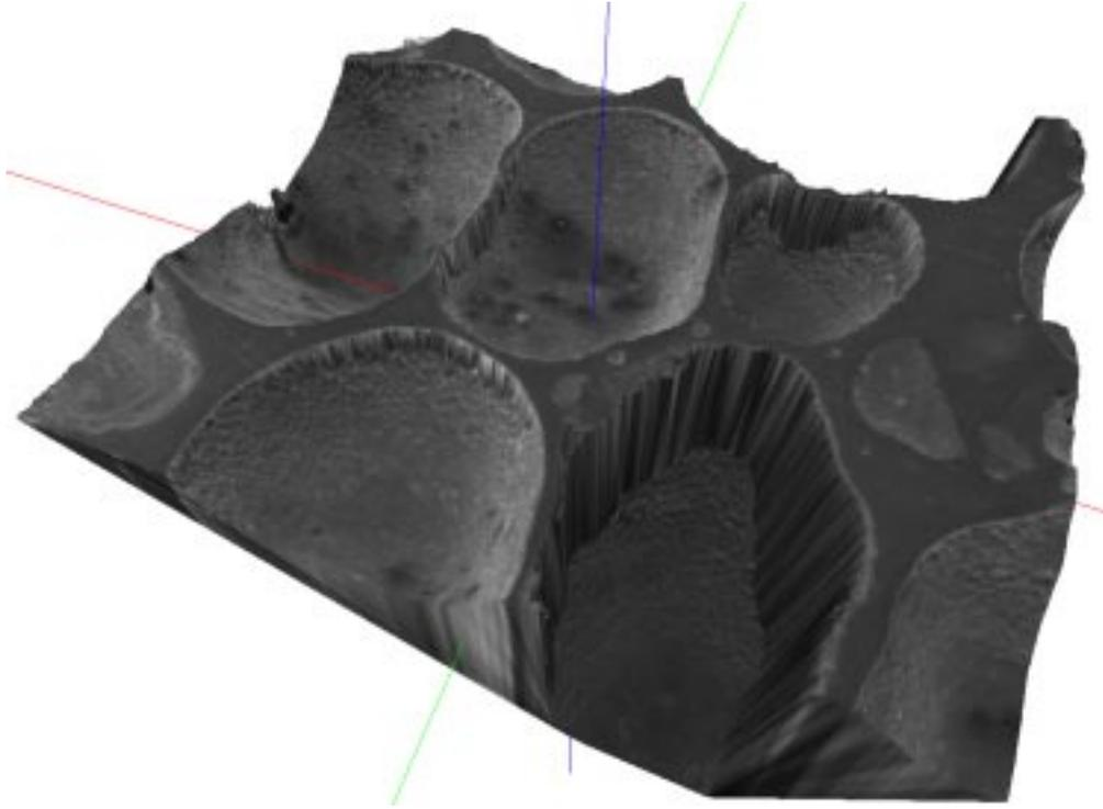
**Figure 3:** Digital elevation model with about 200000 points of a foam surface in front of the notch root.
