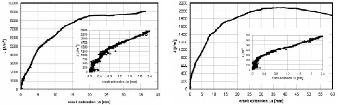
**Figure 4:** J vs.  $\Delta a$  curves of ALPORAS foam CT-specimens ( $W=290$  mm) with two different densities ( $0,49$  g/cm<sup>3</sup> on the left side and  $0,25$  g/cm<sup>3</sup> on the right side).
