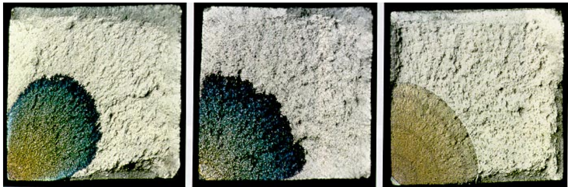
Figure 5: Macrographs of CC specimens tested under (a) 120 s dwell, R=0.1, (b) 120 s dwell, R=0.5, (c) 4 sections of 120 s dwell at 77.5 % of max + 0.25 Hz, R=0.1
