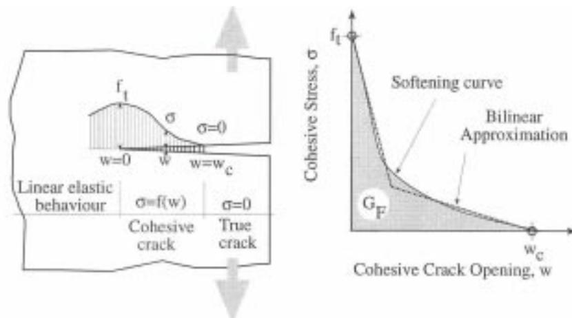
Figure 1: Cohesive crack and softening function.
