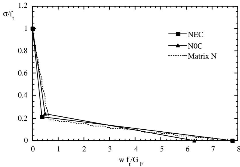
**Figure 6 :** Influence of the interface of crushed aggregates on the softening curve.
