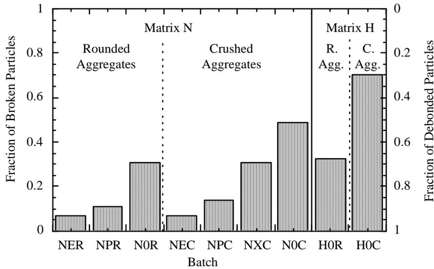
**Figure 2 :** Fraction of broken/debonded particles in the concretes investigated.
