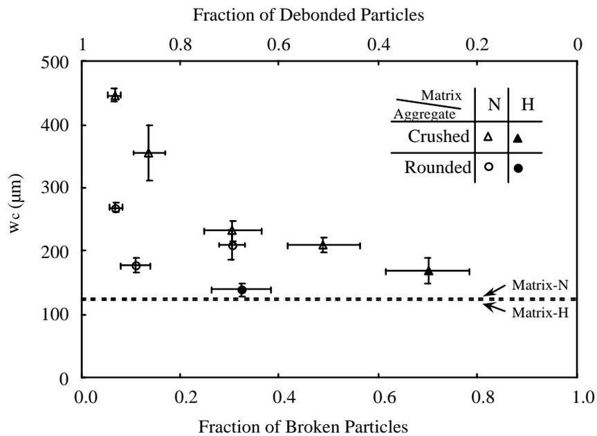
**Figure 5 :** Variation of the critical crack opening with the fraction of broken particles
