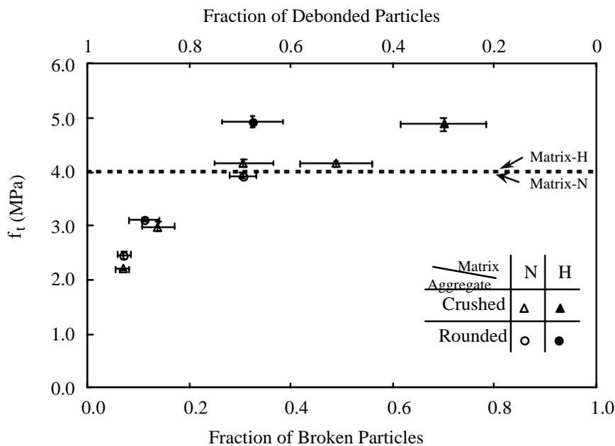
**Figure 3 :** Variation of the tensile strength with the fraction of broken particles
