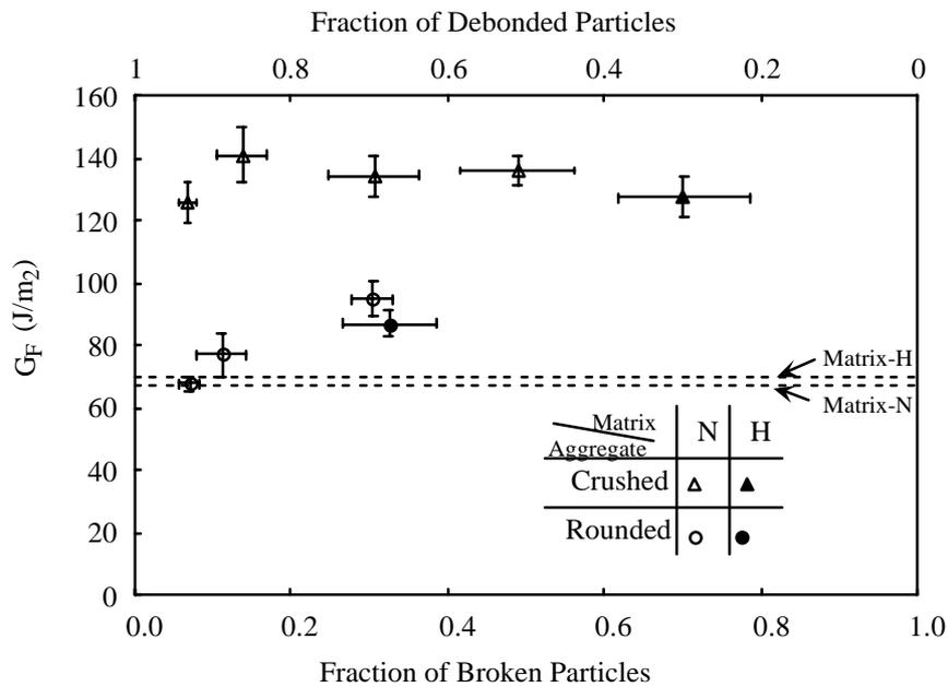
**Figure 4 :** Variation of the fracture energy with the fraction of broken particles
