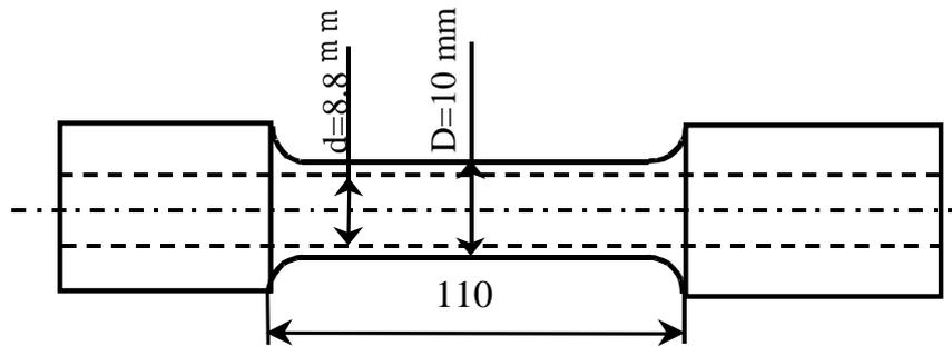
Fig.1c. Specimen geometry for tensile testing of ion nitrided layer.
