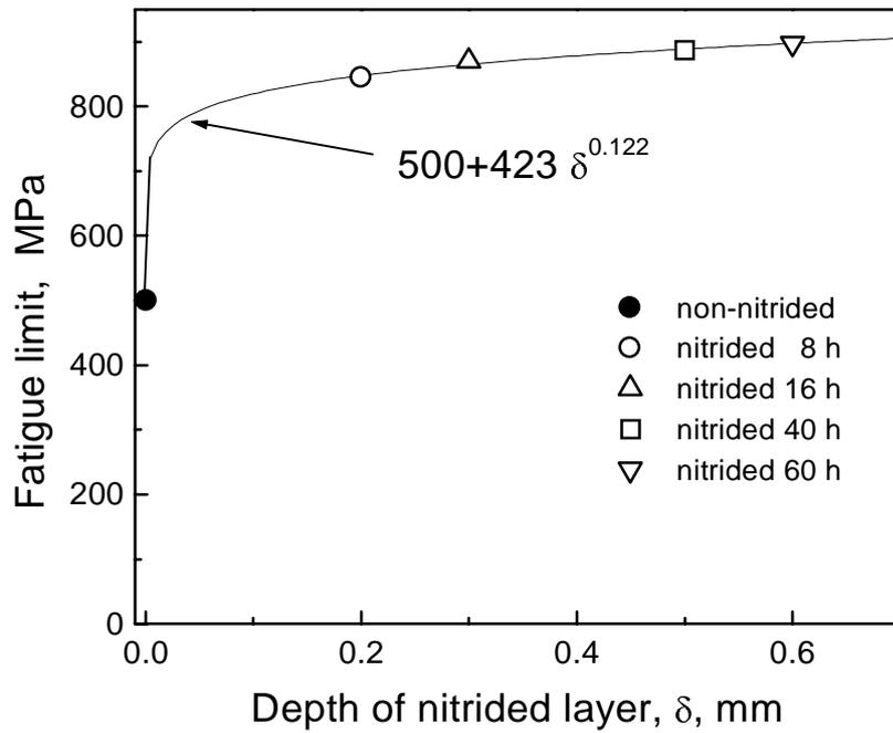
Fig. 3 Variation of fatigue limit with depth of nitrided layer.
