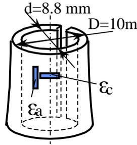
Fig1b. Specimen dimensions after residual stress measurement.
