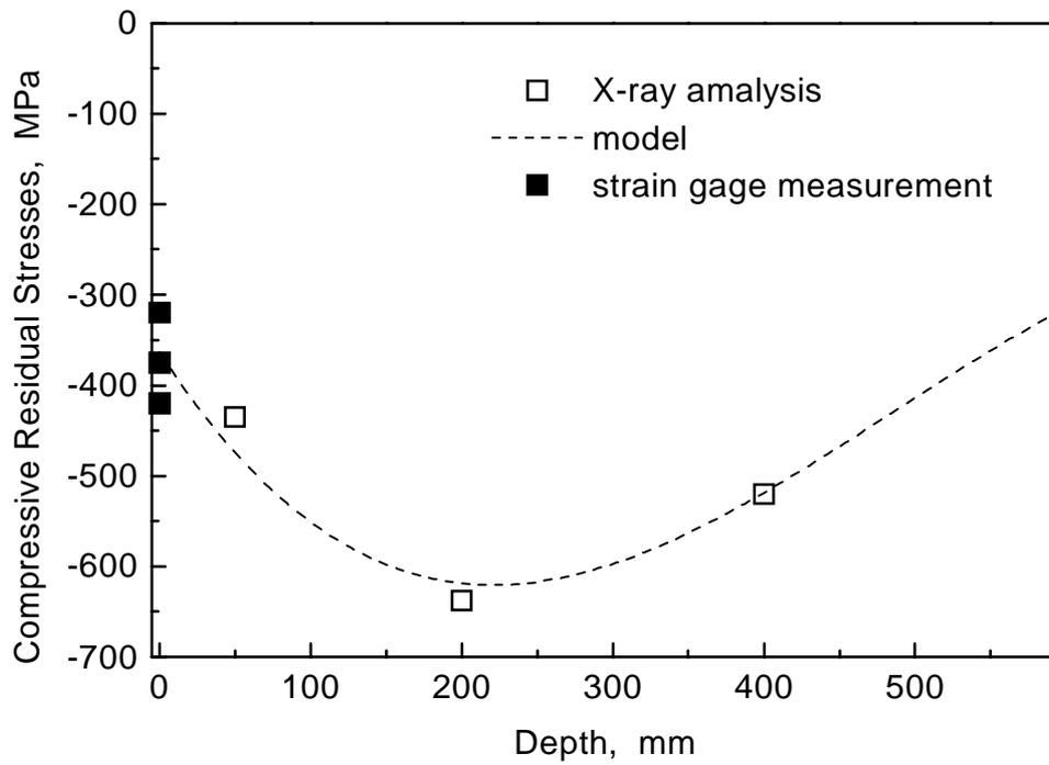
Fig.4. Variation of compressive residual stresses with depth of nitration.
