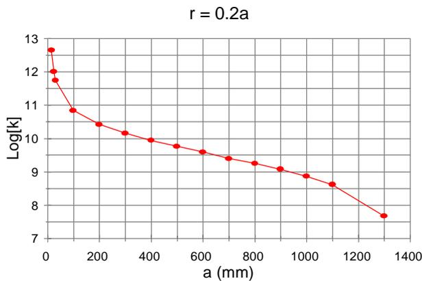
Figure 9: Crack length(a) x flexural stiffness obtained with RAST-  $\xi(a) = r = 0.2a$ .
