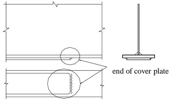
**Figure 1:** Schematic of cover-plated beam showing location of fatigue crack.
