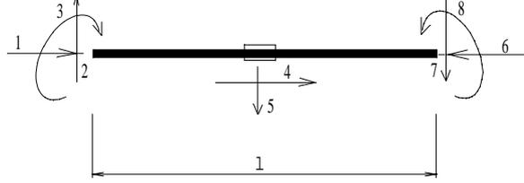
**Figure 5:** Cracked element degrees of freedom.
