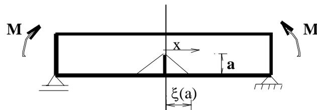
**Figure 2:** Schematic representation of beam with single crack (mode I).
