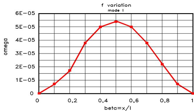
Figure 10: Function  $\Omega(\beta)$  versus position  $\beta=x/L$  for simply supported beam.
