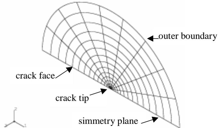
**Figure 1:** Finite element mesh for crack tip problem using element CPE8R.
