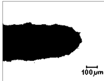
Figure 5: Comparison of the echo amplitude versus load curves and cut views of the specimen AD09. In the left hand photograph mid range graduations are millimetres. In the right hand micrograph we can see the blunting of the crack tip.
