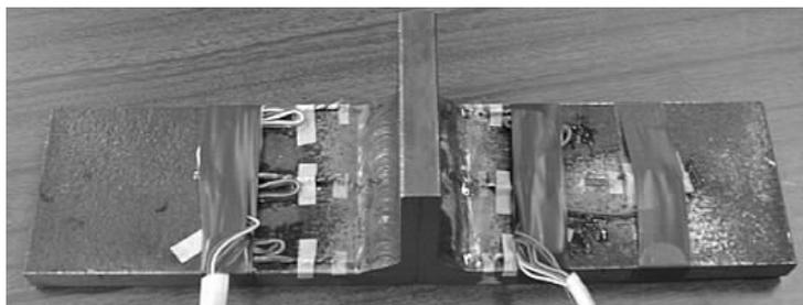
**Fig. 1** - Set-up of the strain gauges used to monitor the onset of crack initiation and detect marking.
