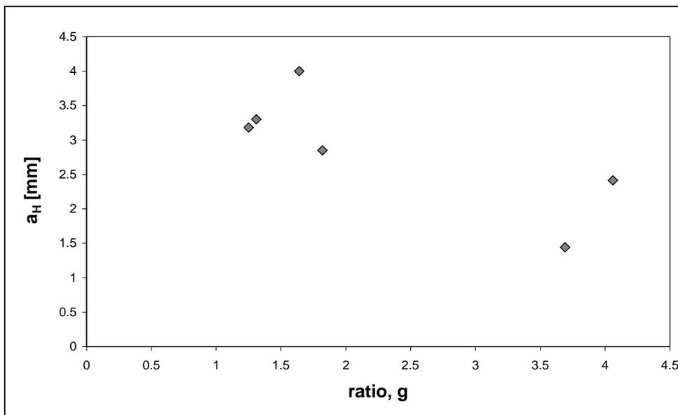
**Fig.6** – Gains in fatigue life due to treatment against depth of the crack repaired by hammer peening. 3PB T non load carrying joint.
