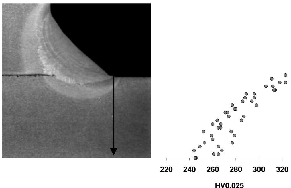
**Fig. 2** - Hardness profiles in the welded joints. c) Hammer peened, microhardness, 25gf.
