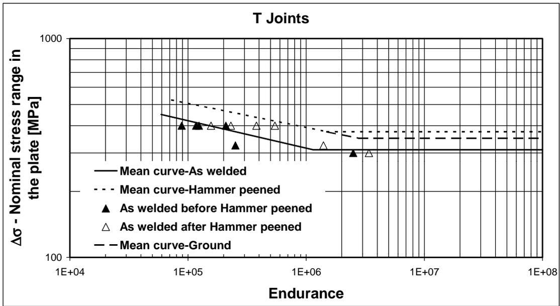
**Fig. 5** - S-N curves of the repaired joints by hammer peening. 3PB T non-load carrying joints. Medium strength St S2-3 steel.
