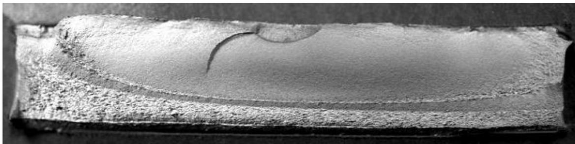
**Fig. 3** - Fatigue fracture surfaces of the 3PB specimens. As welded, followed by hammer peening of a crack of 2.23mm. Fatigue marking at 25% strain reduction.  $\Delta\sigma=325\text{MPa}$ .  $N_i=252406$ .  $N_T=1398259$  cycles.
