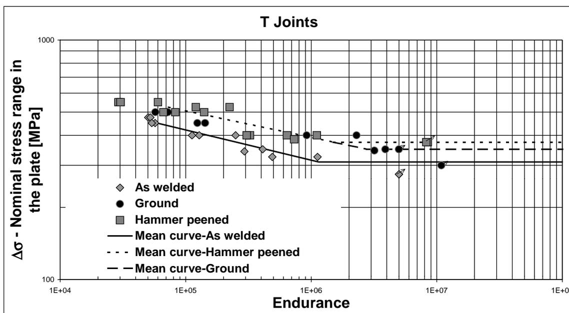
**Fig.4** - S-N curves of the as welded, hammer peened and ground joints. 3PB T non-load carrying joints. St S2-3 steel.
