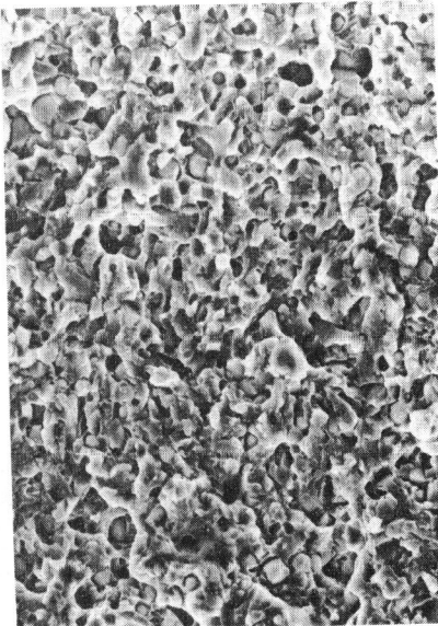
Figure 6 Fracture surface of the PM HS Steel (x 1520)
