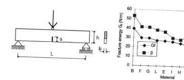
Figure 1 Testing scheme
