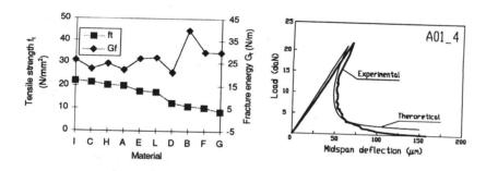
Figure 3 Tensile strength and fracture energy distribution
