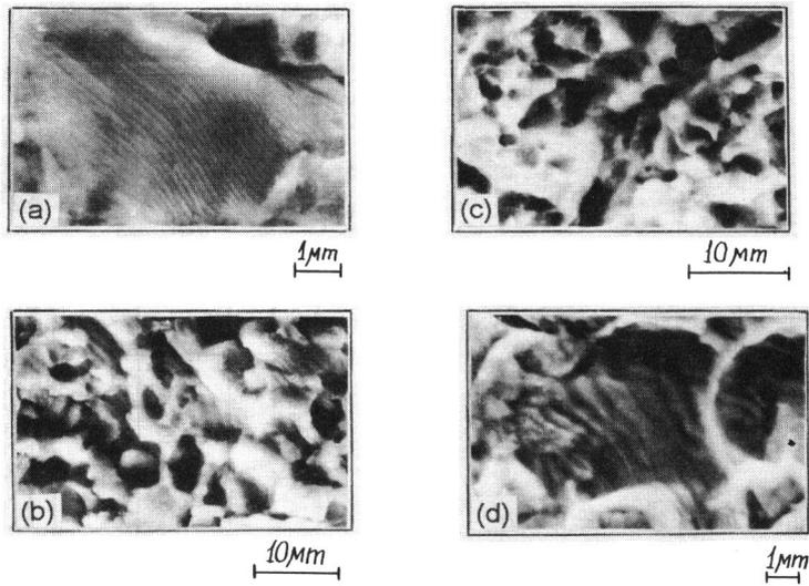
Fig. 2 Microfractograms corresponding to various fracture sections under harmonic loading.
