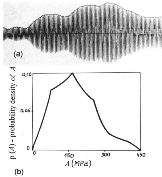
Fig. 3 The MNVS oscillogram and their envelope (a) and the probability density of the envelope (b).
