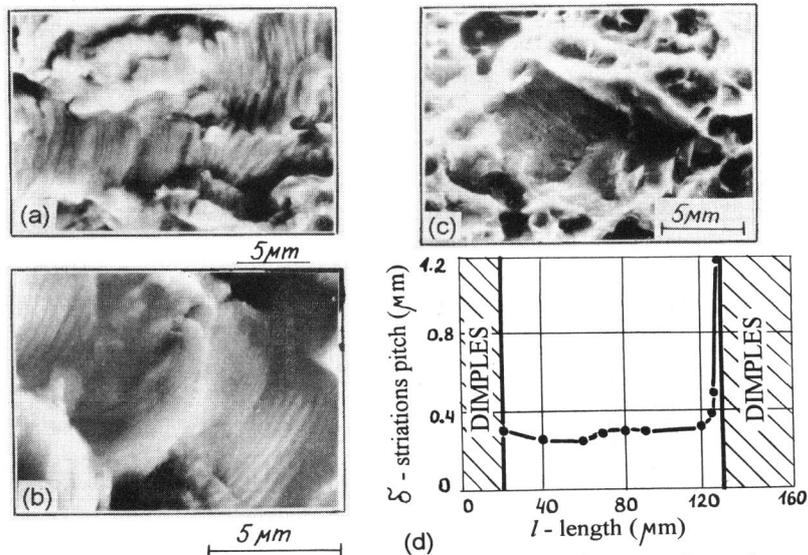
Fig. 4 Microfractograms corresponding to the initial (a,b) and final (c) fracture sections under random loading and change of the striations pitch in the fatigue band (d).
