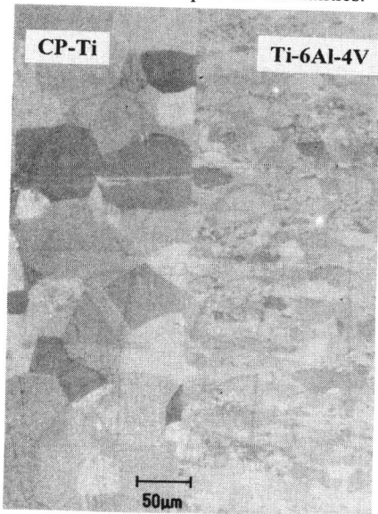
Figure 7 Polarized light micrograph showing the bond line
