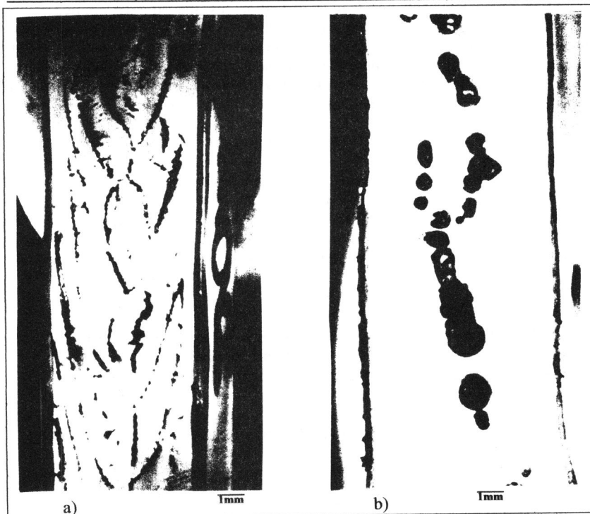
Fig. 2 Damage obtained during explosive decompression tests (10MPa; 100°C) a) 1 minute decompression: cracks b) 1 hour decompression: bubbles.
