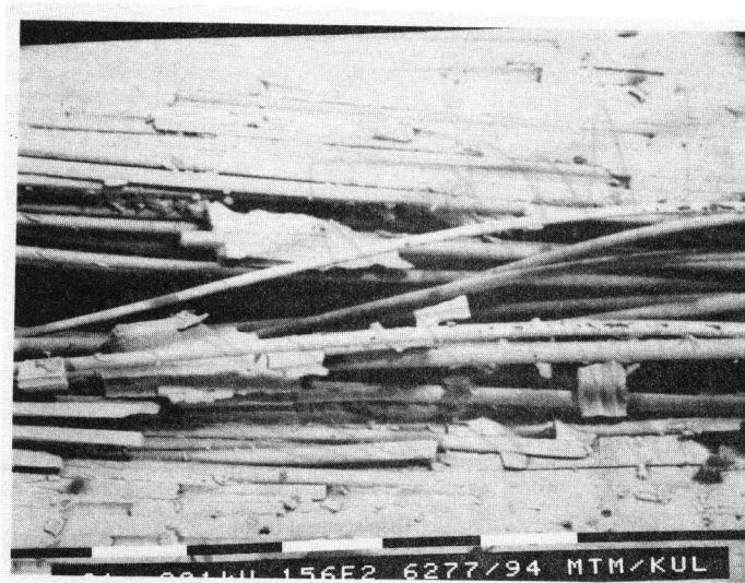
Figure 4 : Crack bridging by intact fibres
