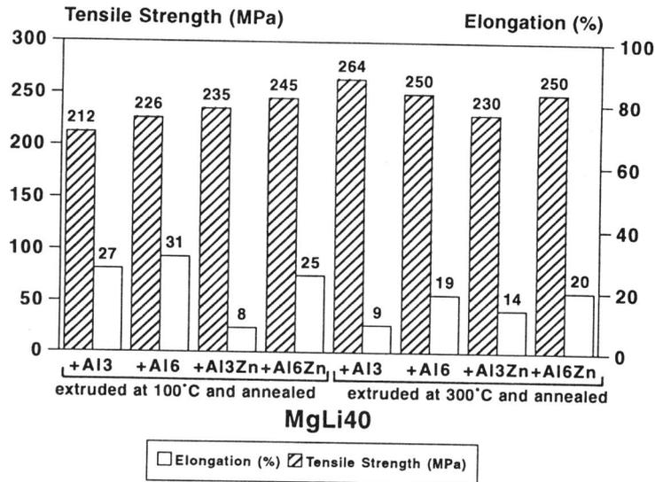
Figure 1 Tensile strength and elongation of investigated alloys (2)
