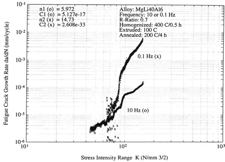
Figure 5 Effect of frequency on crack growth rate
