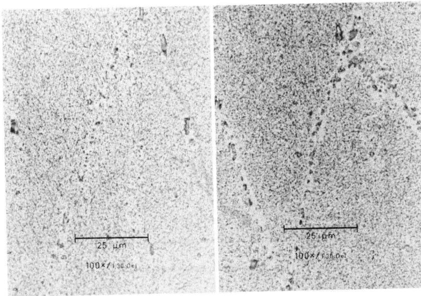
Figure 3 Mg-Li40Al6 extruded at 100°C      Mg-Li40Al6 extruded at 300°C
