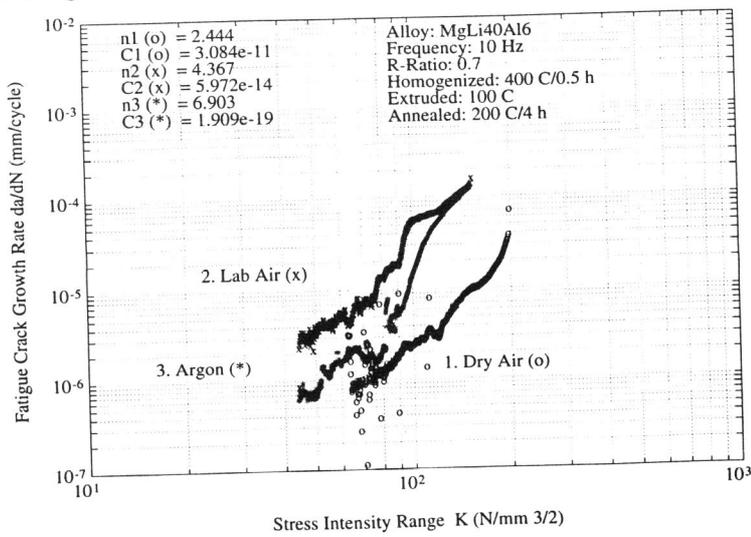
Figure 4 Influence of environments on the stable crack growth
