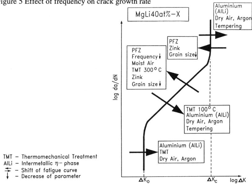
Figure 6 Microstructural effects on stable crack growth of Mg-Li40at%-X-alloys
