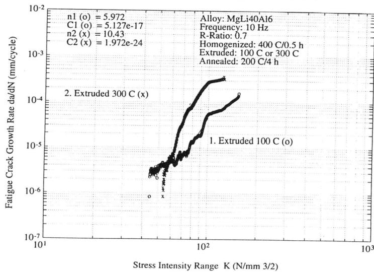
Figure 2 Influence of thermomechanically treatment on Mg-Li40Al6 alloys
