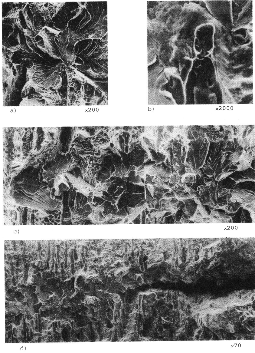
Figure 1. Damage accumulation near sulphide tips in the pipe 1 (a,b- embrittled zone, c- zones coalescence, d- crack initiation)
