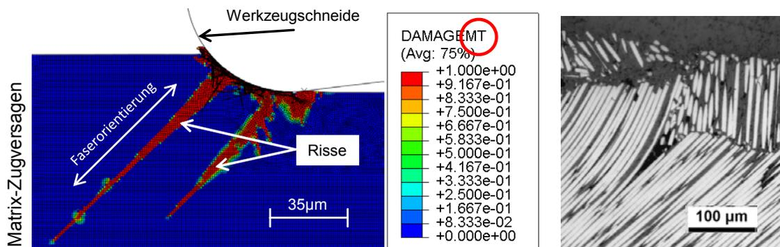
Figure 8. Main CFRP damage for -45° fiber orientation by matrix tensile failure (left, macroscopic model) and its respective experimental observation (right)
