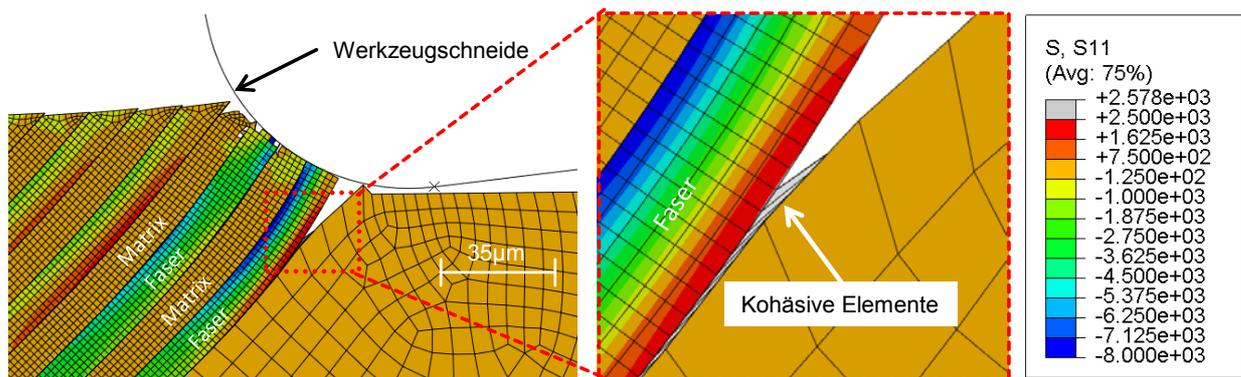
Figure 9. Longitudinal fiber stress just before fiber failure and fiber/matrix interface failure for  $-45^\circ$  fiber orientation (microscopic model)
