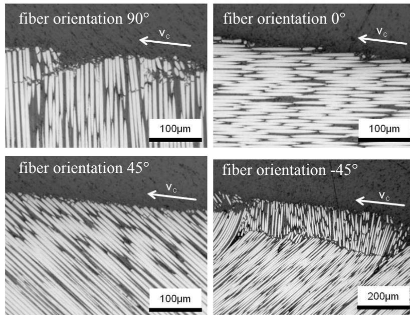
Figure 2. Micrographs of specimens with different fiber orientations
