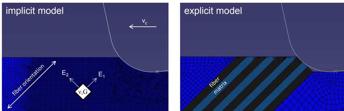
Figure 4. Setups of an implicit macroscopic and an explicit microscopic FEM model for the CFRP cutting simulation
