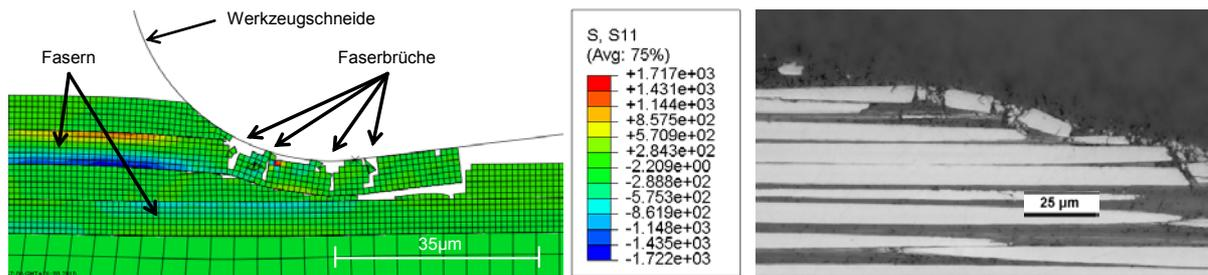
Figure 5. Horizontal stress and damage for  $0^\circ$  fiber orientation (microscopic model)
