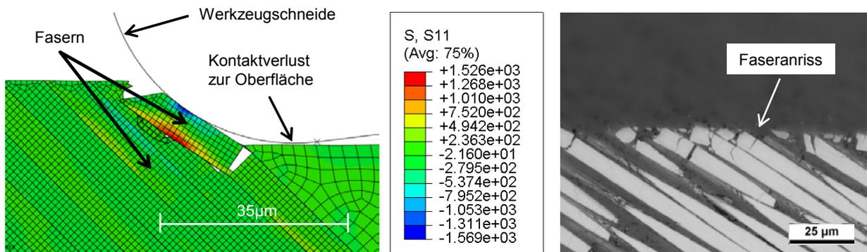
Figure 7. Longitudinal fiber stress and damage for +45° fiber orientation (microscopic model) and its respective experimental observation (right)
