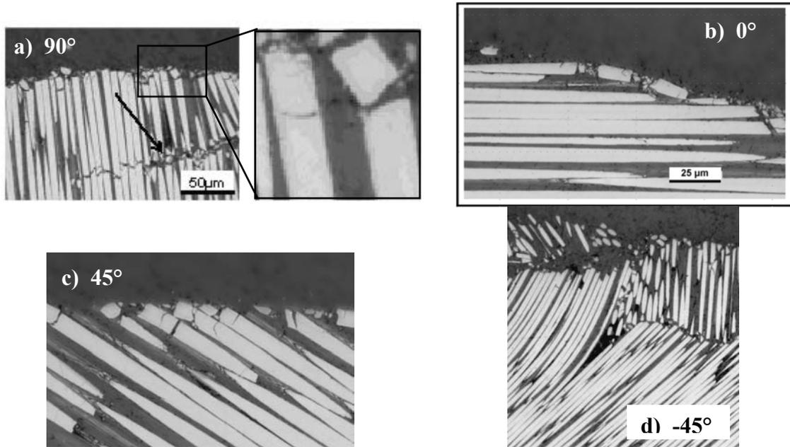
Figure 3. CFRP fiber / matrix microstructures at bottom of milled slots in specimens with different fiber orientation (cutting from right to left)
