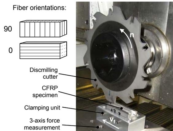
Figure 1. Experimental setup for slot milling in unidirectional CFRP with fiber orientation  $0^\circ$ ,  $45^\circ$ ,  $-45^\circ$  and  $90^\circ$
