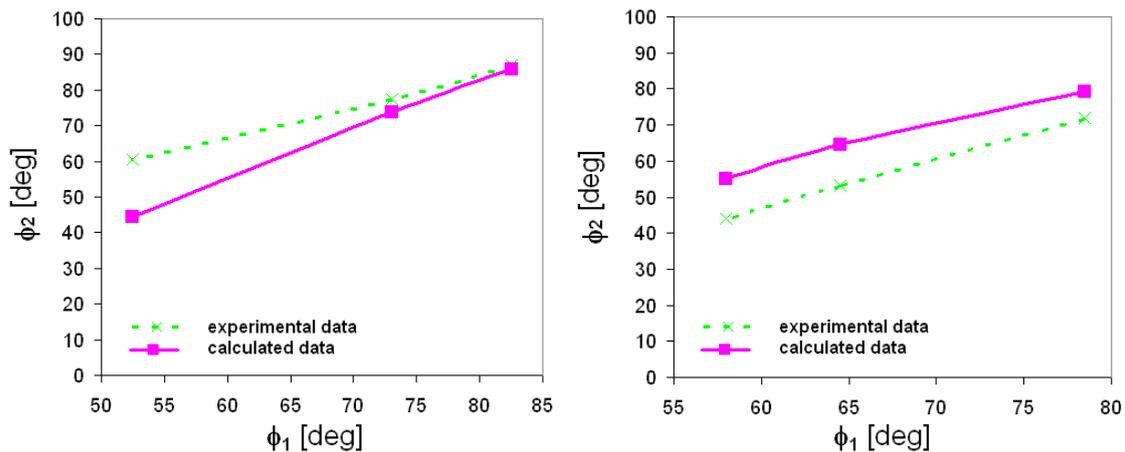
Figure 7. Further crack propagation direction behind the bimaterial interface: comparison of calculated values and experimental data ( $\text{Al}_2\text{O}_3/\text{ZrO}_2$  interface on the left;  $\text{ZrO}_2/\text{Al}_2\text{O}_3$  on the right)
