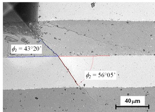
Figure 2. Change of crack propagation direction at interface between two materials. The crack was induced by indentation – by courtesy of H. Hadraba
