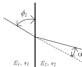
Figure 5. Scheme of crack propagation after its pass through bimaterial interface
