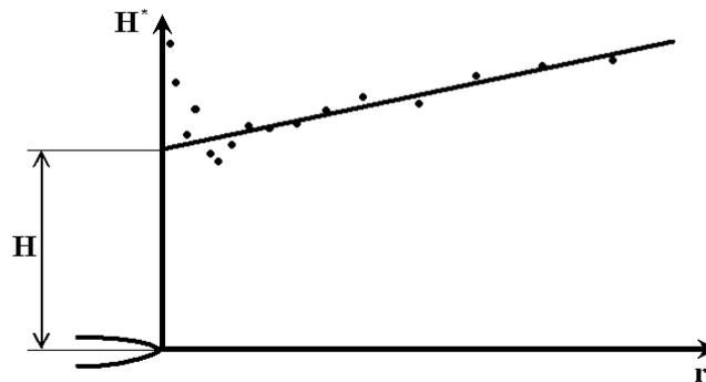
Figure 6. Procedure of  $H_I, H_{II}$  determination: linear extrapolation of  $H(r)$  values for  $r=0$
