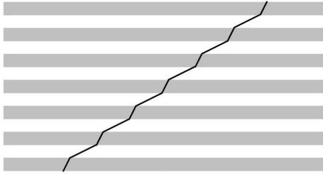
Figure 1. Scheme of stepwise crack propagation through ceramic laminate
