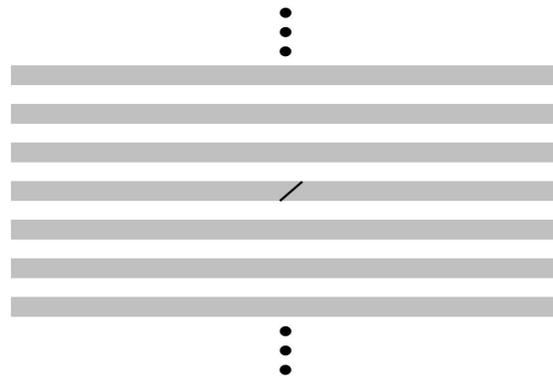
Figure 3. Scheme of numerical model: layered ceramics with initial internal crack with tips at material interfaces
