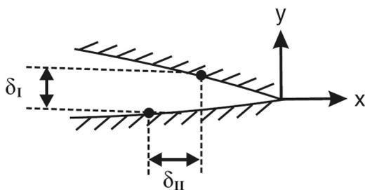
Figure 4. Displacements  $\delta_I, \delta_{II}$  at the crack tip
