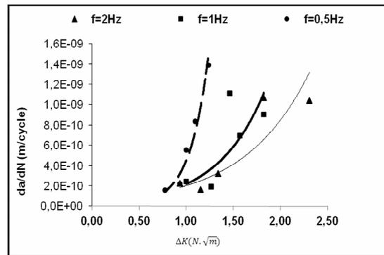
Figure 10. Crack growth rate according stress intensity factor.
