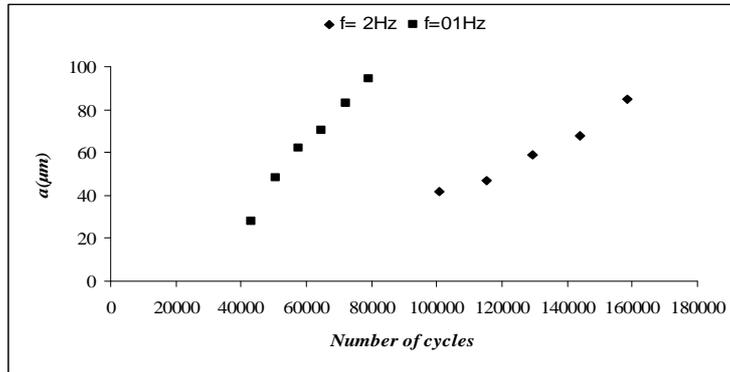
Figure9. Effect of the stress frequency on the evolution of crack size.
