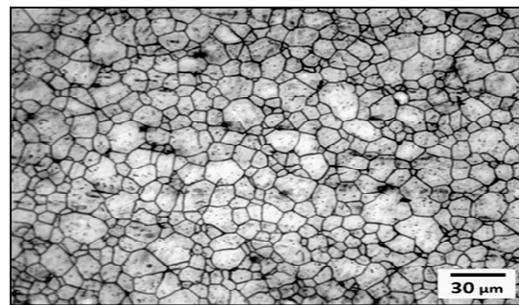
Figure.2: Microstructure of 316L stainless steel with enlarging of 650
