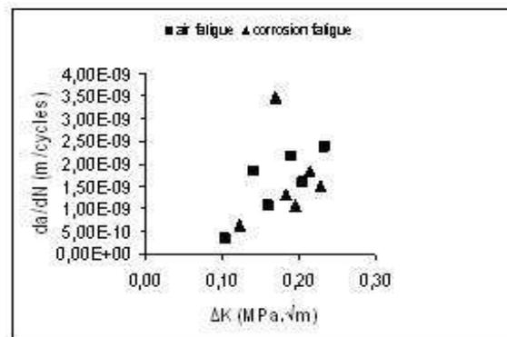
Figure.6: Propagation rate of cracks for the fatigue corrosion.
