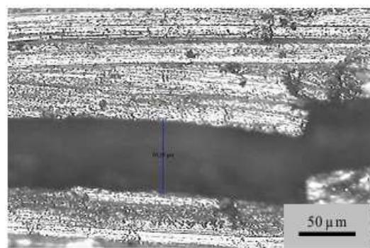
Figure 4. Crack propagation of aluminium alloy
