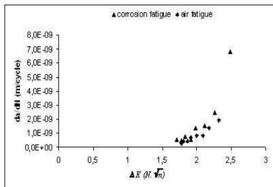
Figure 8. Crack growth rate according stress intensity factor
