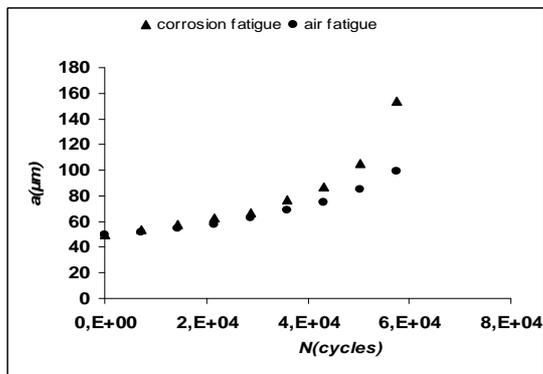
Figure 7. Evolution of crack size according to the number of cycles.
