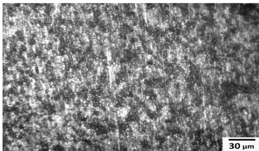
Figure.1: Microstructure of AW2024 with enlarging of 650.
