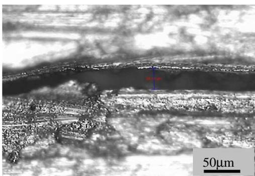
Figure 3. Initiation cracks on aluminium alloy
