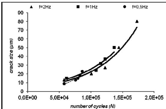
Figure 9. Evolution of crack size according number of cycles.
