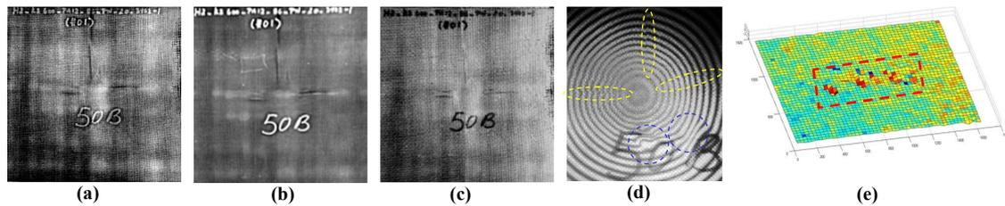
Figure 2. 50B Kevlar impacted specimen. *Front side inspection*: (a) PPT phasegram  $f=0.22$  Hz, (b) 3<sup>rd</sup> empirical orthogonal function by PCT, (c) HOS, 5<sup>th</sup> moment reconstructed image, (d) HI-DE result ( $t_{exp}=1s$ ), (e) DSP, Surf result using MatPIV 1.6.1
