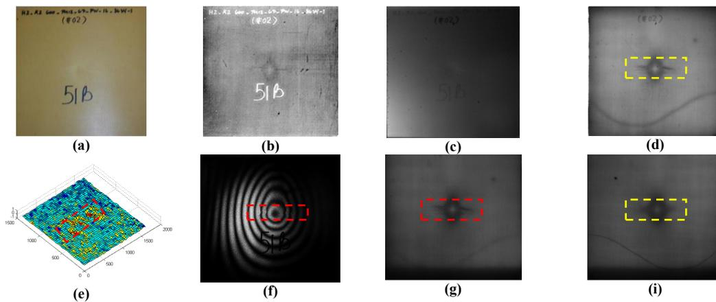
Figure 3. 51B Kevlar impacted specimen. *Front side inspection*: (a) photograph, (b) 5<sup>th</sup> empirical orthogonal function by PCT, (c) NIR reflectogram using filter (Camera Mutech), (d) NIR transmittogram using a filter (Camera Mutech), (e) DSP, Surf result using MatPIV 1.6.1, (f) HI-DE result ( $t_{exp}=1s$ ), (g) NIR transmittogram using a wide spectrum source (Camera Goodrich), *Back side inspection*: (i) NIR transmittogram using a wide spectrum source (Camera Goodrich)
