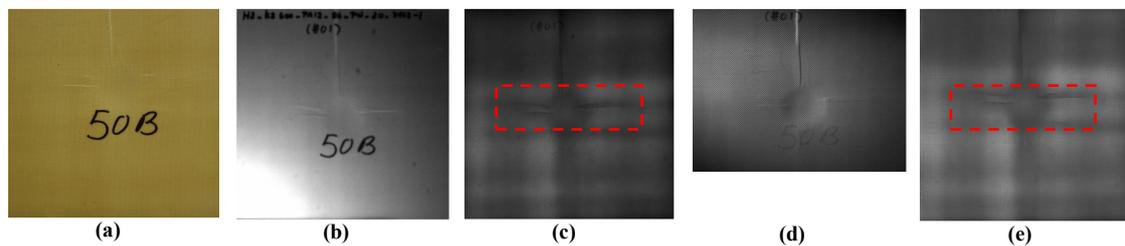
Figure 1. 50B Kevlar impacted specimen inspected with a CCD camera. *Front side inspection*: (a) photograph, (b) NIR reflectogram using filter (Camera Mutech), (c) NIR transmittogram using a wide spectrum source (Camera Mutech), (d) NIR reflectogram using a 940 nm source (camera Goodrich), (e) NIR transmittogram using a wide spectrum source (Camera Goodrich)
