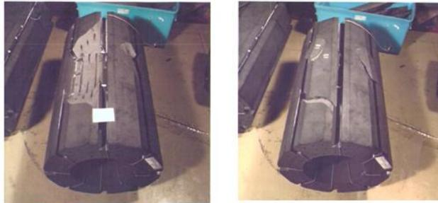
Figure 5. Crack path on the third test case.
