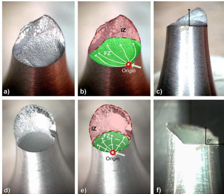
Figure 4. **Loading case PT**: fracture surface for a), b) 42CrMo4 and d) e), Mg AZ31B-F. Crack initiation angle for c) 42CrMo4 and f) Mg AZ31B-F.
