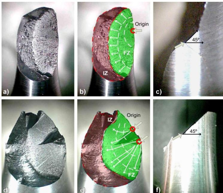
Figure 5. **Loading case PS**: fracture surface for a), b) 42CrMo4 and d) e), Mg AZ31B-F. Crack initiation angle for c) 42CrMo4 and f) Mg AZ31B-F.
