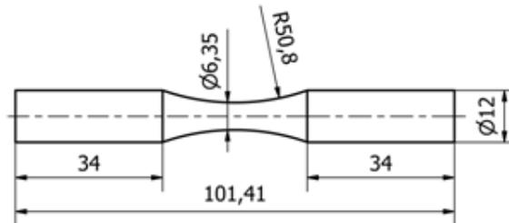
Figure 2. Specimen test geometry and dimensions (mm).
