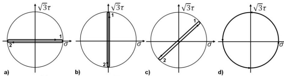
Figure 1. Loading path: a) case PT, b) case PS, c) case PP and d) case OP.
