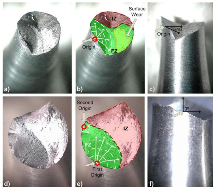
Figure 6. **Loading case PP:** fracture surface for a), b) 42CrMo4 and d) e), Mg AZ31B-F. Crack initiation angle for c) 42CrMo4 and f) Mg AZ31B-F.
