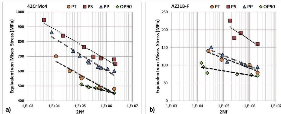
Figure 3. SN curves for: a) 42CrMo4 and b) Mg AZ31B-F.
