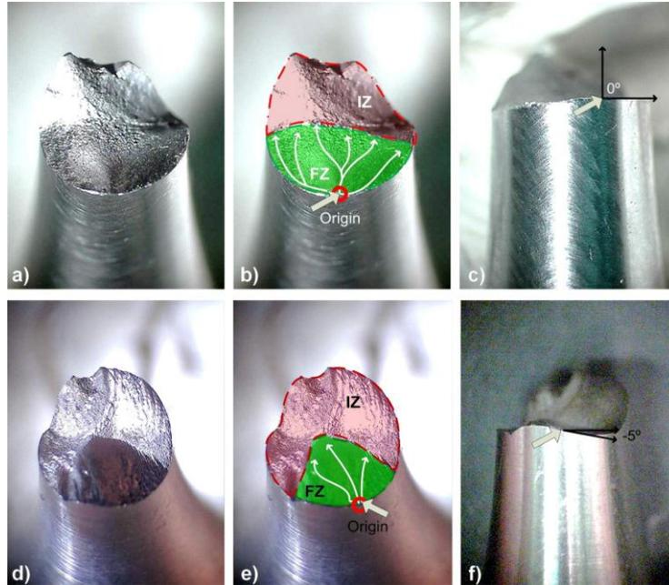
Figure 7. **Loading case OP:** fracture surface for a), b) 42CrMo4 and d) e), Mg AZ31B-F. Crack initiation angle for c) 42CrMo4 and f) Mg AZ31B-F.
