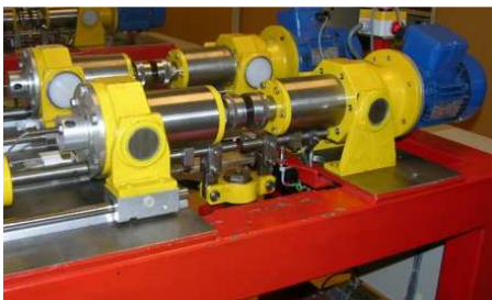
Fig. 1 Conventional rotating bending machine for high cycle fatigue (HCF) tests designed by AMB (Chair of Mechanical Engineering)
