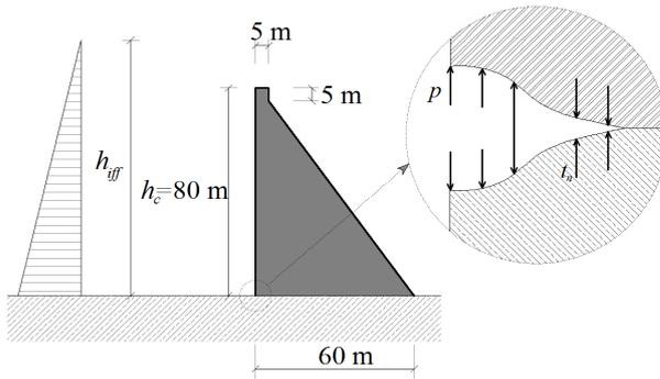
Figure 3. Gravity dam proposed as benchmark by ICOLD [9].
