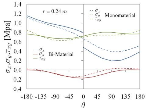
Figure 4. First term ( $\lambda \leq 1.5$ ) of the asymptotic expansion: comparison between the monomaterial case and bi-material case
