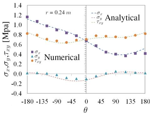
Figure 5. Comparison between an analytical ( $\lambda \leq 1.5$ ) and numerical solution in the monomaterial case
