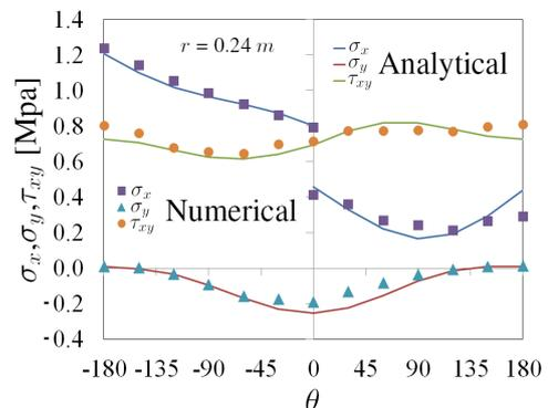
Figure 6. Comparison between an analytical ( $\lambda \leq 1.5$ ) and numerical solution in the bi-material case
