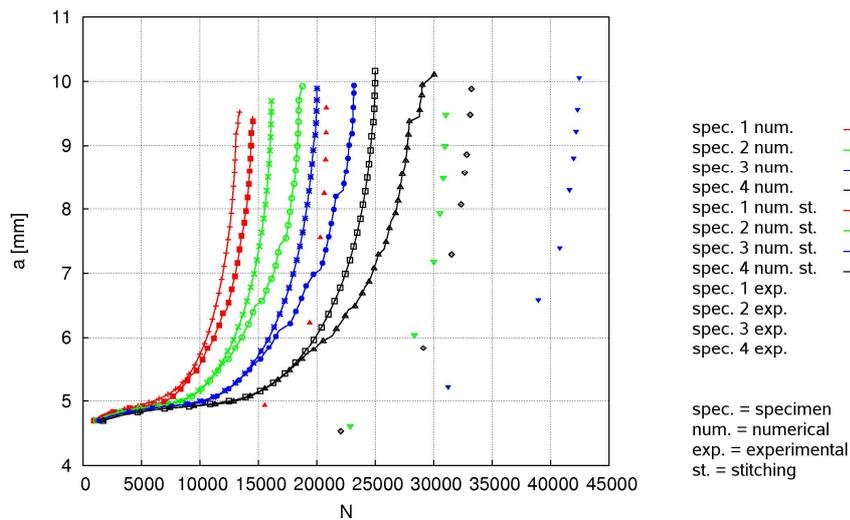
Figure 7. Crack propagation for the 4PB-Specimen.
