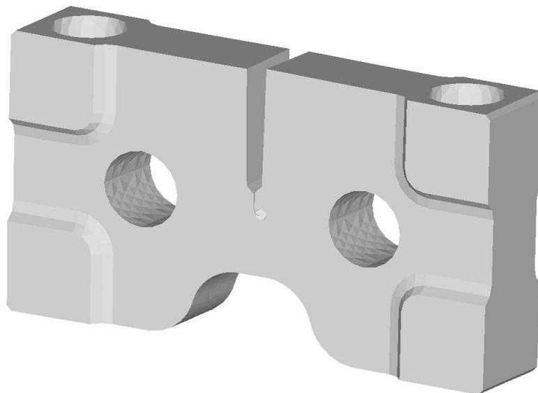
Figure 8. Compact Tension Shear Rotation Specimen.
