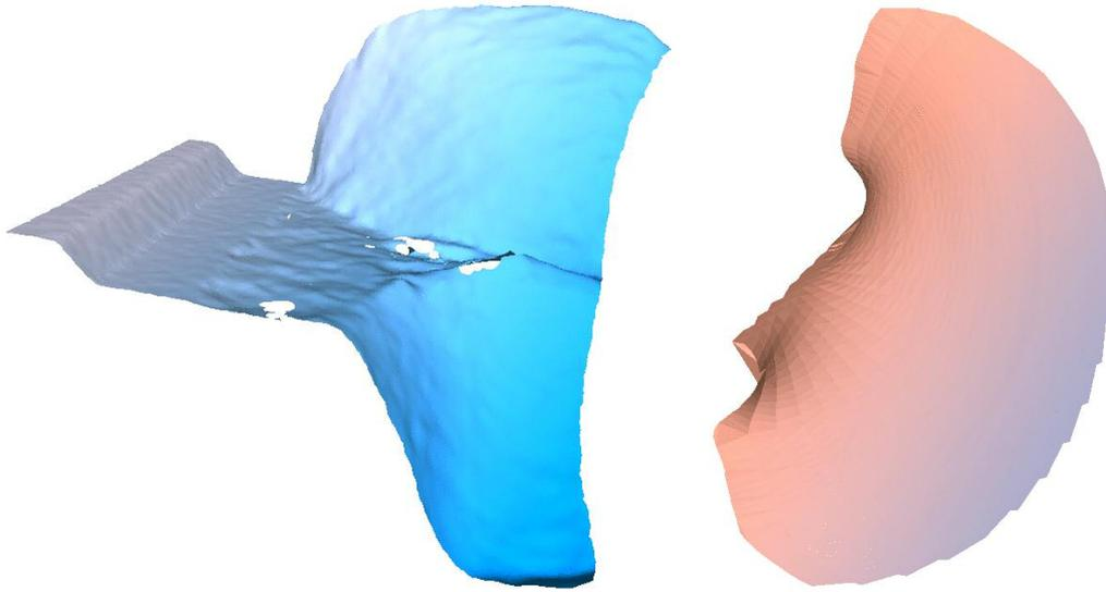
Figure 9. Experimental (left) and numerical (right) crack shape for the CTSR-Specimen.
