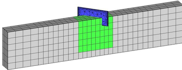
Figure 4. Initial crack (blue), domain (green) and rest (gray) for the 4PB-specimen.
