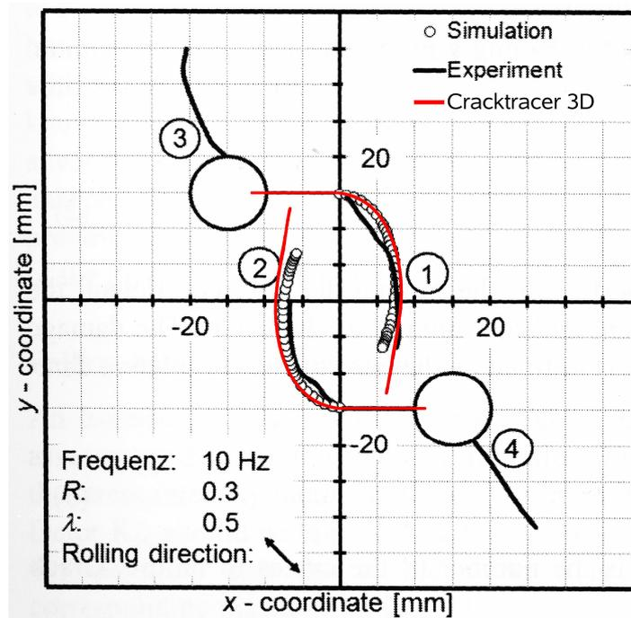
Figure 10. Crack propagation in a biaxial plate.
