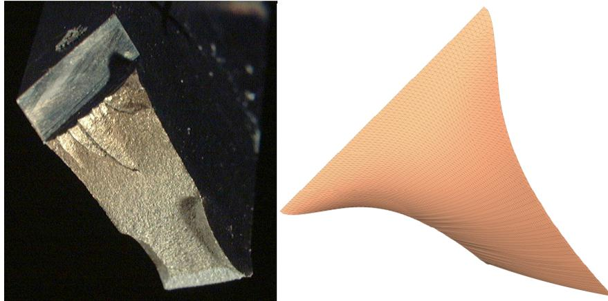
Figure 6. Crack shape (left: experimental; right: numerical) in the 4PB-Specimen.
