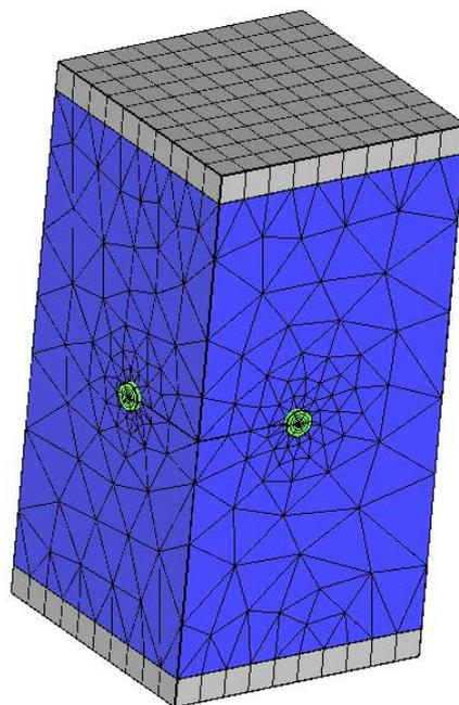
Figure 1. Tube (green), domain (blue) and original mesh (gray) for the CC-Specimen.
