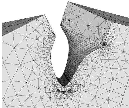
Figure 5. Crack propagation in the 4PB-Specimen.
