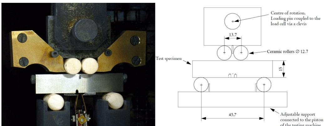
Figure 3. Experimental set-up of the 4PB tests.
