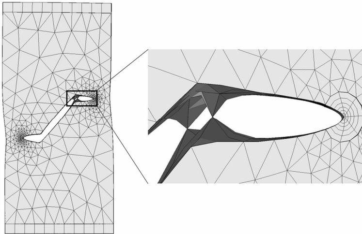
Figure 2. Stitching in the CCT-Specimen.
