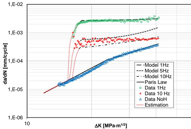
Figure 4: X65 steel: model prediction and experimental data at  $T = 23\text{ }^{\circ}\text{C}$ .
