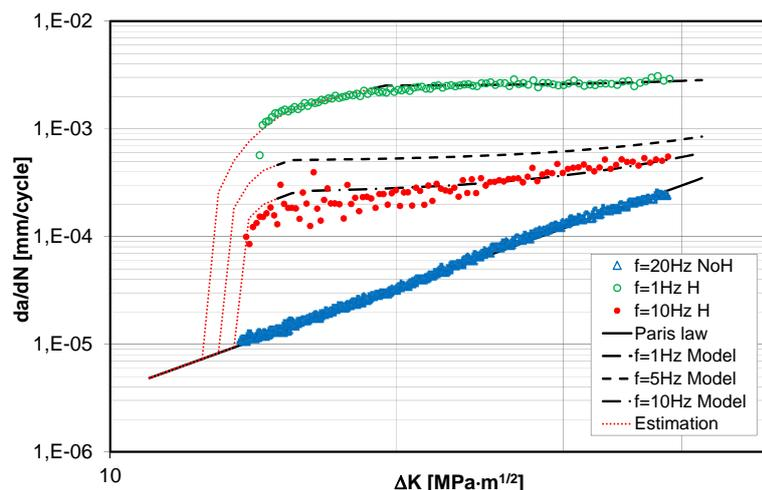
Figure 2: F22 steel: model prediction and experimental data at  $T = 23^{\circ}\text{C}$ .
