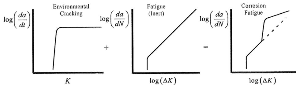
Figure 1. Schematisation of the superposition model [13].
