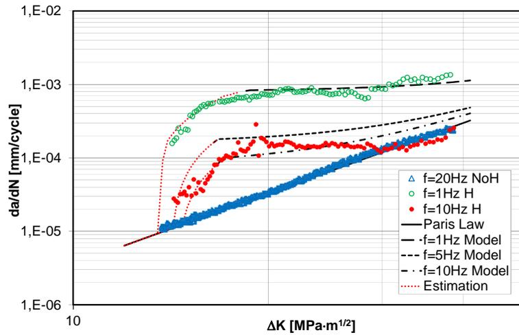
Figure 3: F22 steel: model prediction and experimental data at  $T = -30\text{ }^{\circ}\text{C}$ .
