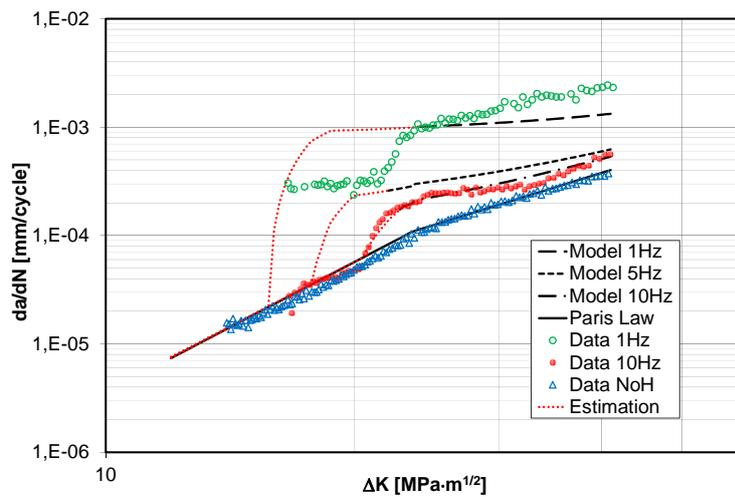
Figure 5: X65 steel: model prediction and experimental data at  $T = -30\text{ }^{\circ}\text{C}$ .
