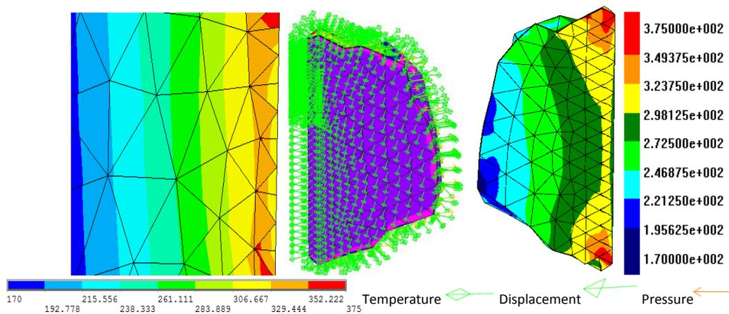
Figure 9. FEM (left) and DBEM (right) maximum principal stress in the subdomain, with highlight of boundary conditions on the DBEM subdomain boundaries (centre).
