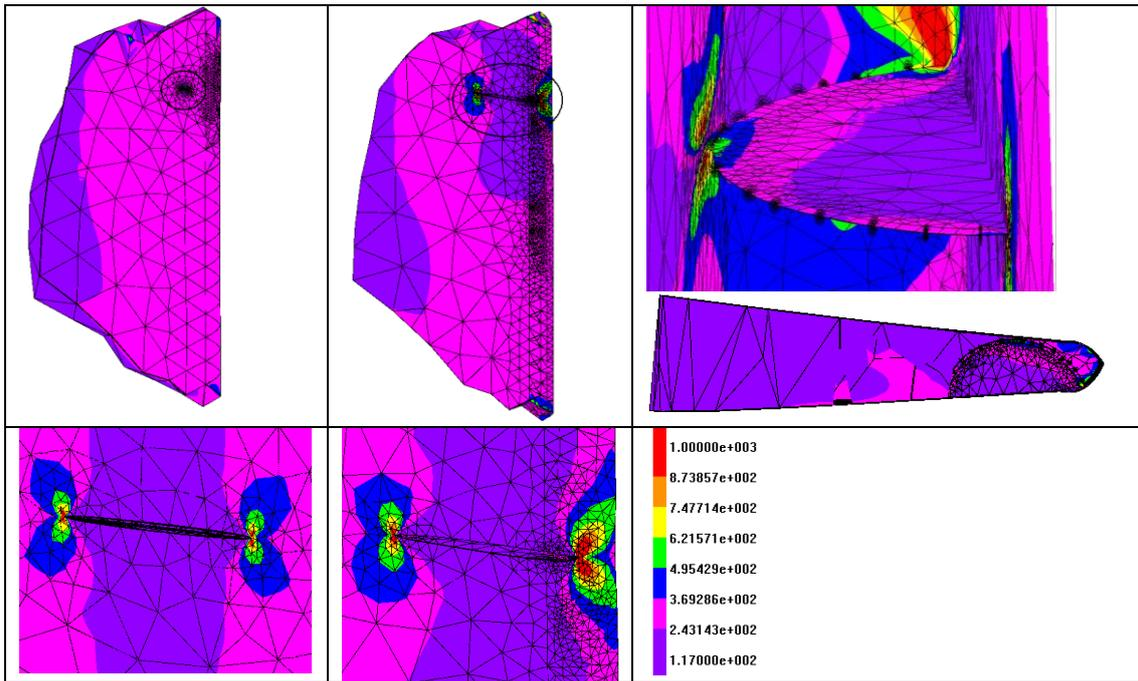
Figure 10. Von Mises stresses (MPa) on the initial (left) and final cracked configuration (middle), with an internal view of the crack that is becoming through the thickness.
