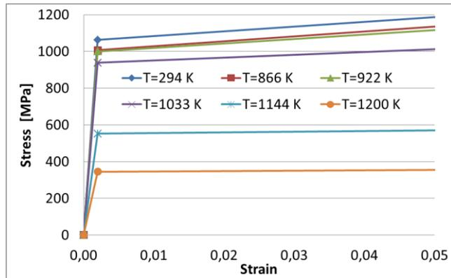
Figure 3. Stress-strain curves vs. temperatures.
