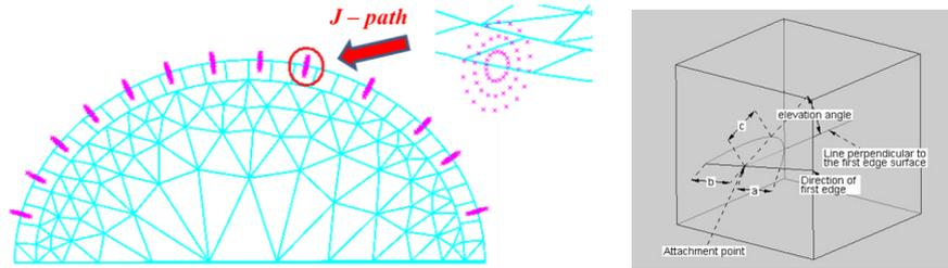
Figure 6. Initial crack mesh with highlight of the j-path along the crack front, needed for the j-integral evaluation (left); scheme showing the crack introduction procedure (right).
