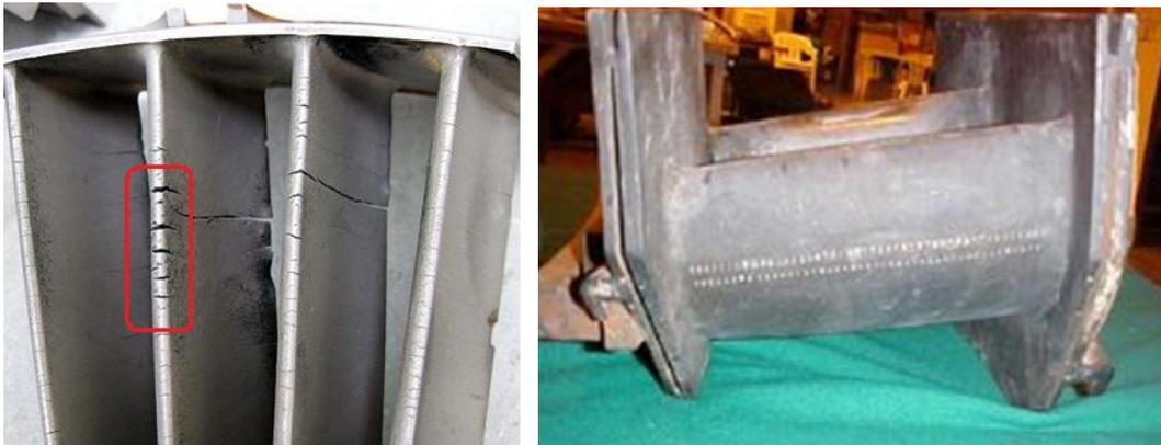
Figure 1. NGV stress rupture cracking. Figure 2. NGV with highlight of cooling holes.
