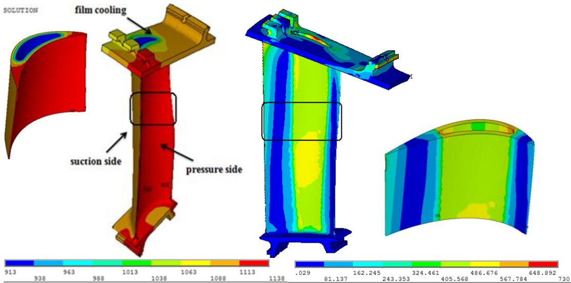
Figure 8. Distribution of temperatures (K) (left) and Von Mises stresses (right) with close-up of the FEM volume where to extract the cracked subdomain.
