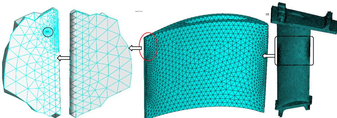
Figure 5. From right to left: overall FEM mesh, FEM sub-volume with refined mesh, DBEM extracted submodel, DBEM mesh refinement after crack insertion.
