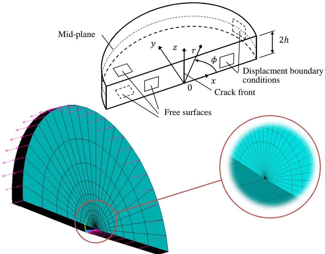
Figure 2. Finite element model geometry and boundary conditions
