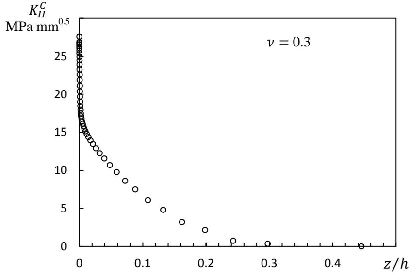
Fig.4b The dependence of the singular coupled mode,  $K_{II}^C$ , across the plate thickness for  $h = 10$  mm and  $c_1 = 1$  MPa mm<sup>-0.5</sup>
