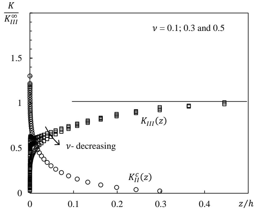
Fig.3b The dependence of the intensity of the primary (mode II)  $K_{III}(z)$  and the coupled mode  $K_{II}^c(z)$  across the plate thickness in the area near the crack tip. The influence of Poisson's ratio on the intensity of the coupled mode is very weak and results are not shown for the sake of the clarity of the figure.
