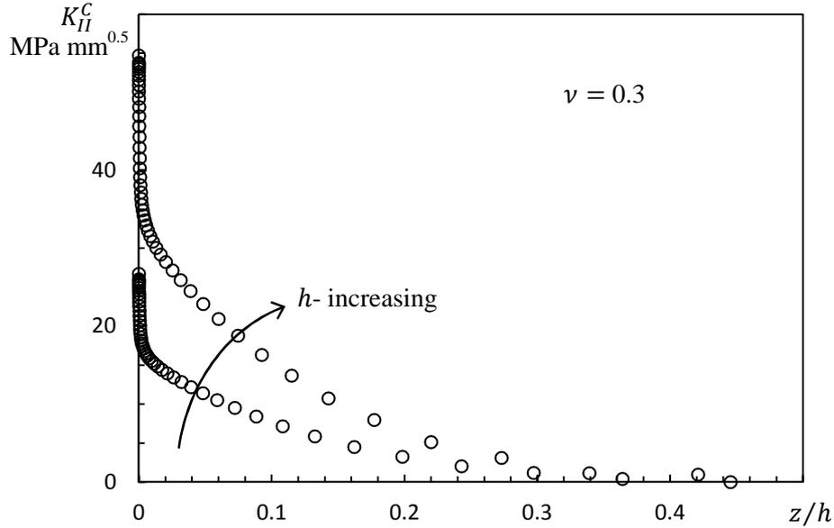
Fig.5. Intensities of the coupled modes for two different plate thicknesses  $h = 10$  and  $20$  mm ( $c_1 = 1 \text{ MPa mm}^{-0.5}$ )
