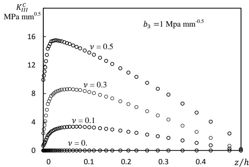
Fig.4a The dependence of the singular coupled mode,  $K_{III}^C$ , across the plate thickness for  $h = 10$  mm and  $b_3 = 1$  MPa mm<sup>-0.5</sup>
