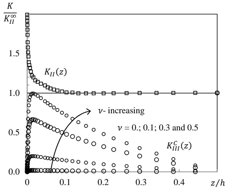
Fig.3a The dependence of the intensity of the primary (mode II)  $K_{II}(z)$  and the coupled mode  $K_O(z) = K_{III}^c(z)$  across the plate thickness in the area near the crack tip. The influence of Poisson's ratio on the intensity of the primary mode is very weak and results are not shown for the sake of the clarity of the figure.
