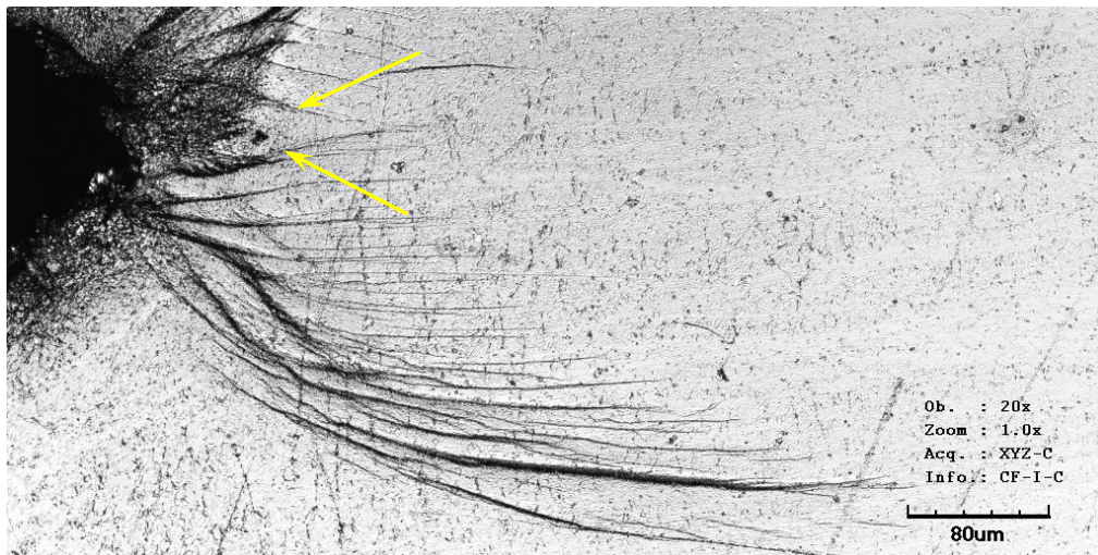
Figure 3. 3D CLSM image showing the lower half of a set of shear bands at the crack tip in PC, with the innermost shear bands marked with the arrows.
