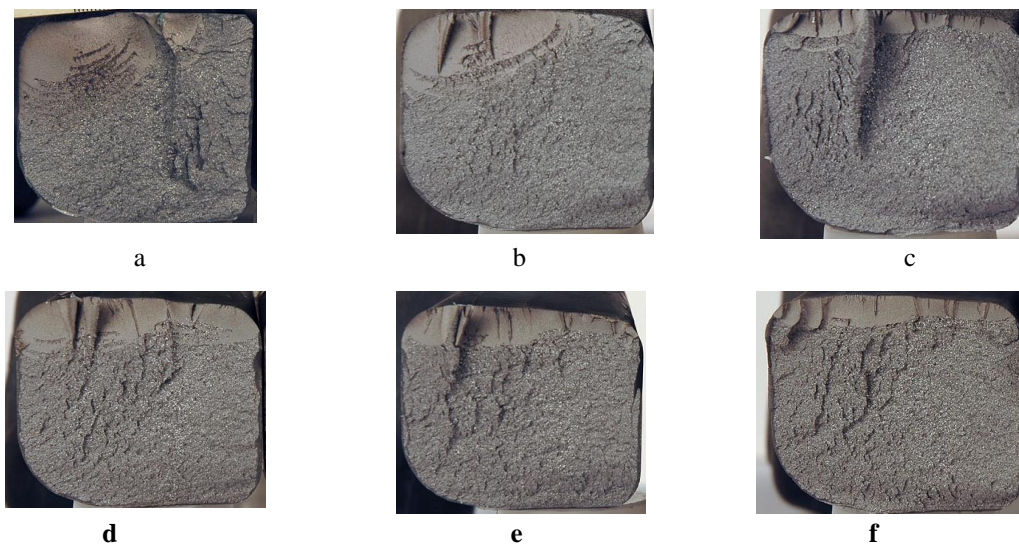
Figure 9: Variable loading fracture surfaces; Shot blasted and tested at maximum load a) 50 kN, b) 55 kN, c) 70 kN and as forged, tested at maximum load d) 45 kN, e) 50 kN and f) 55 kN.
