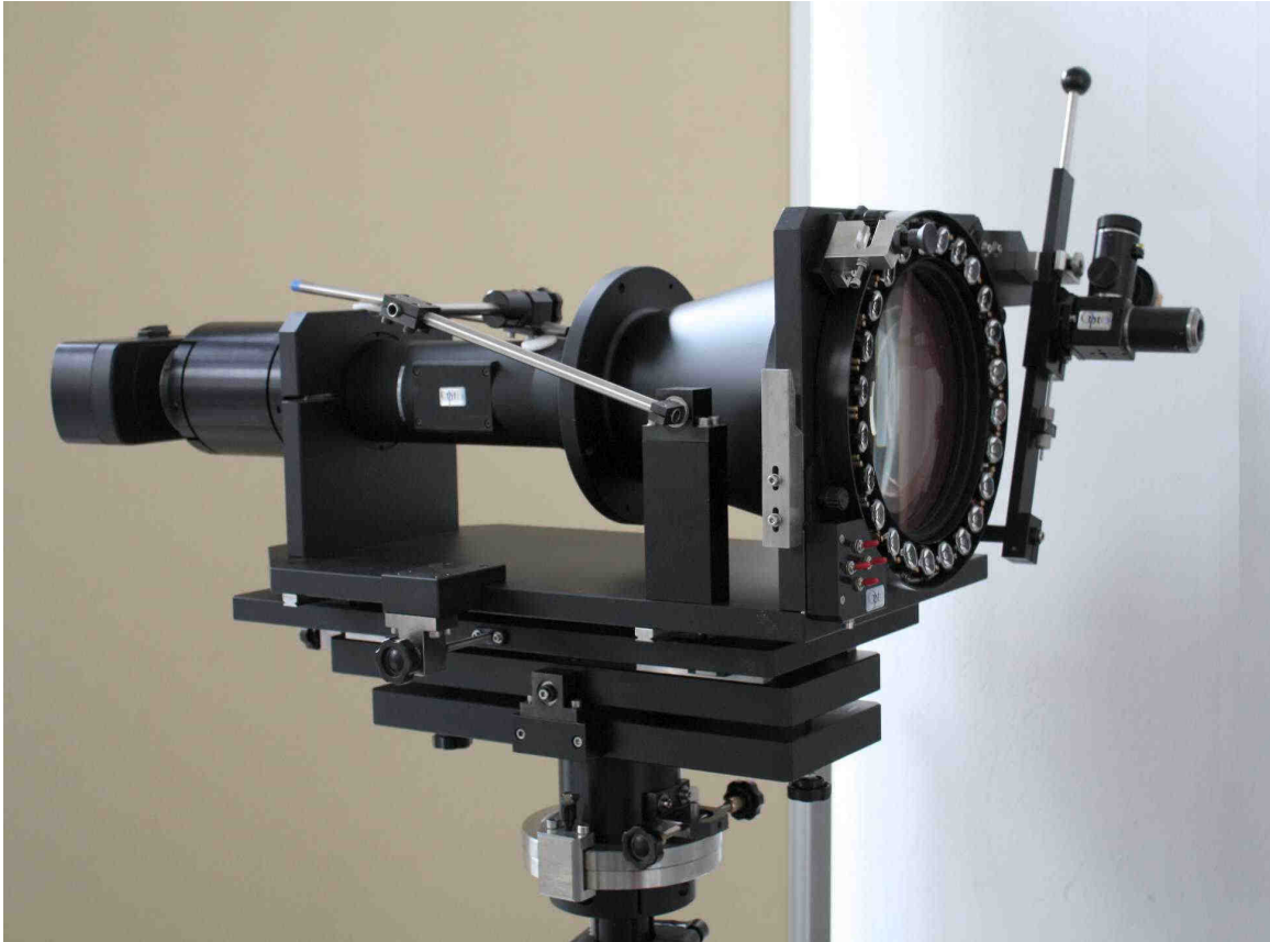
Figure 8. Scanner camera system consists of: Pentaccon scan 6000, telecentric lens, LED ring light and alignment kit
