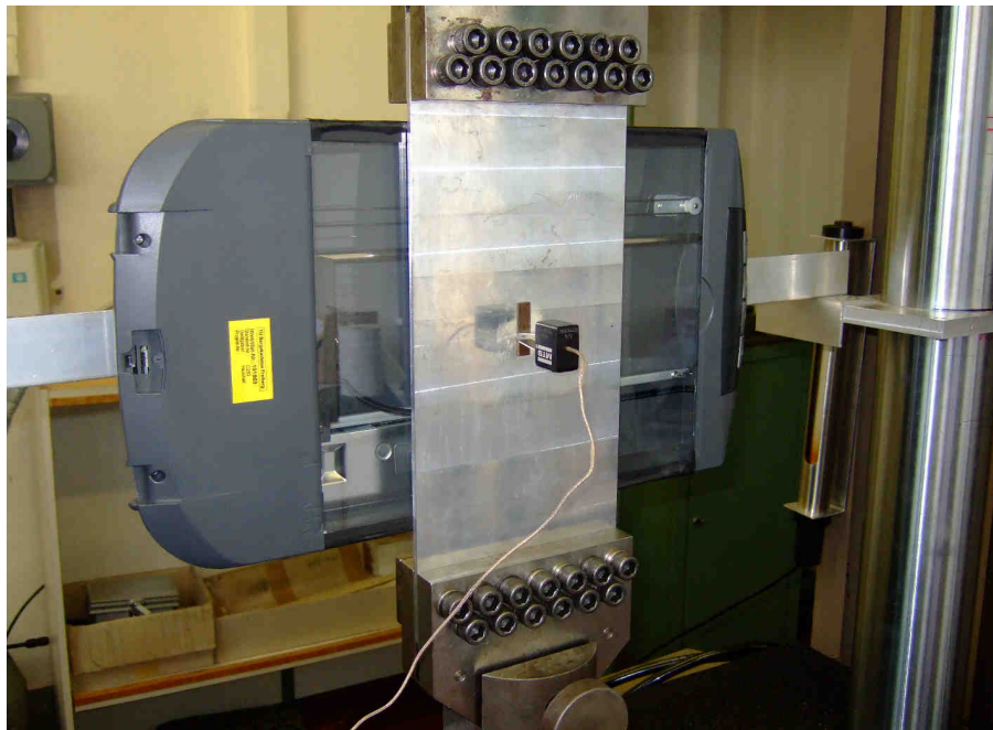
Figure 1. Test set-up with modified flatbed scanner and 160 mm CCT-sample
